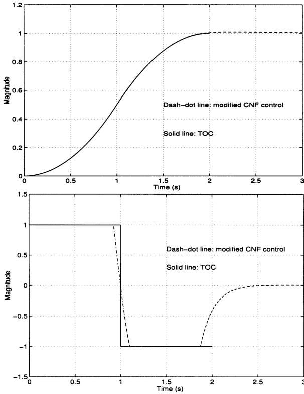
Fig. 2. Responses and control signals of the TOC and CNF control.
