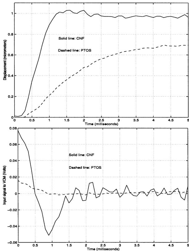
Fig. 8. Experimental result: responses under CNF and PTOS control for  $SL = 1 \mu\text{m}$ .
