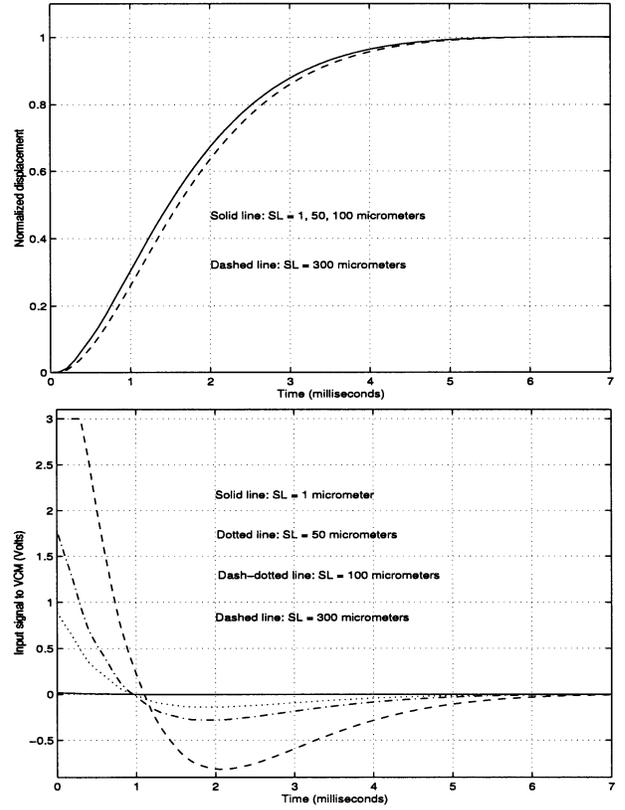
Fig. 7. Simulation result: normalized responses under the PTOS control.
