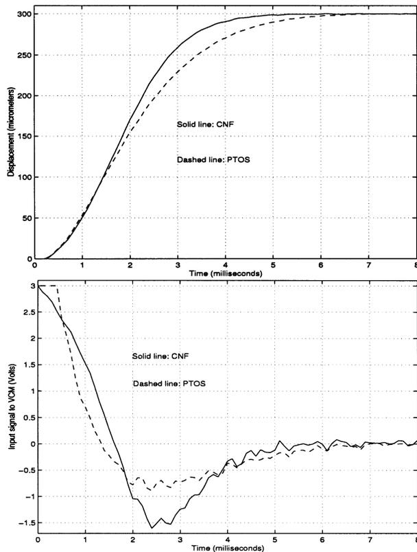
Fig. 10. Experimental result: responses under CNF and PTOS control for  $SL = 300 \mu\text{m}$ .
