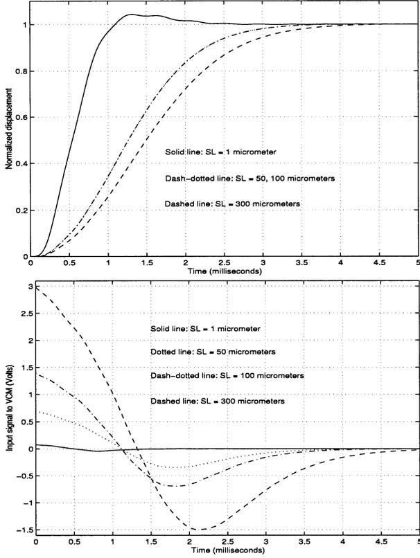
Fig. 6. Simulation result: normalized responses under the CNF control.
