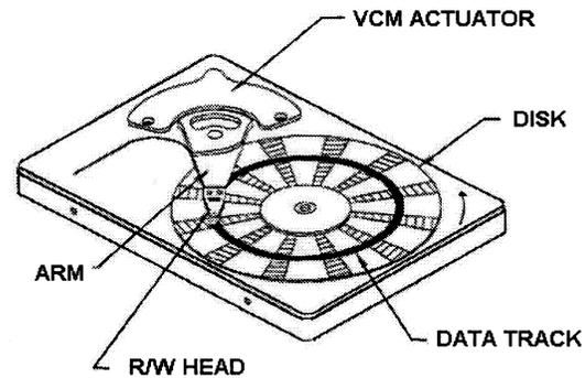
Fig. 4. A typical HDD with a VCM actuator.
