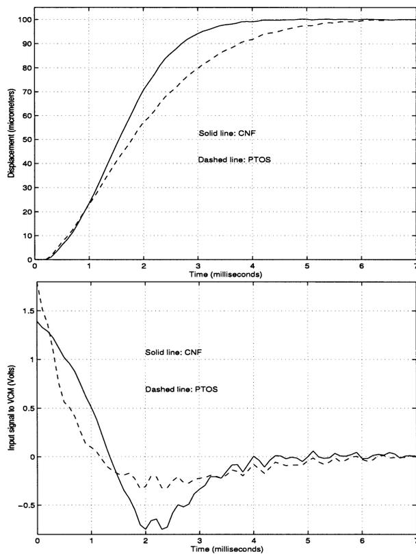
Fig. 9. Experimental result: responses under CNF and PTOS control for  $SL = 100 \mu\text{m}$ .
