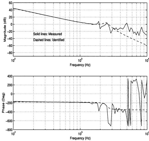
Fig. 5. Frequency response of the HDD.
