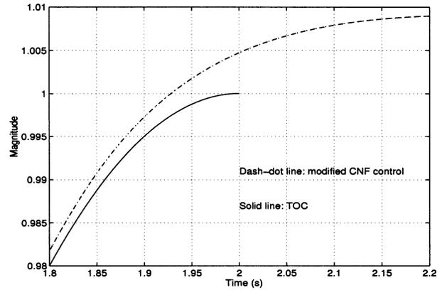
Fig. 3. Controlled output responses around the target reference.
