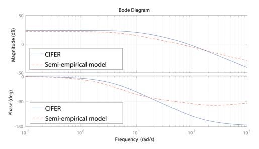
Fig. 19. Comparison of bode plots from CIFER and semi-empirical model for thrust channel.
