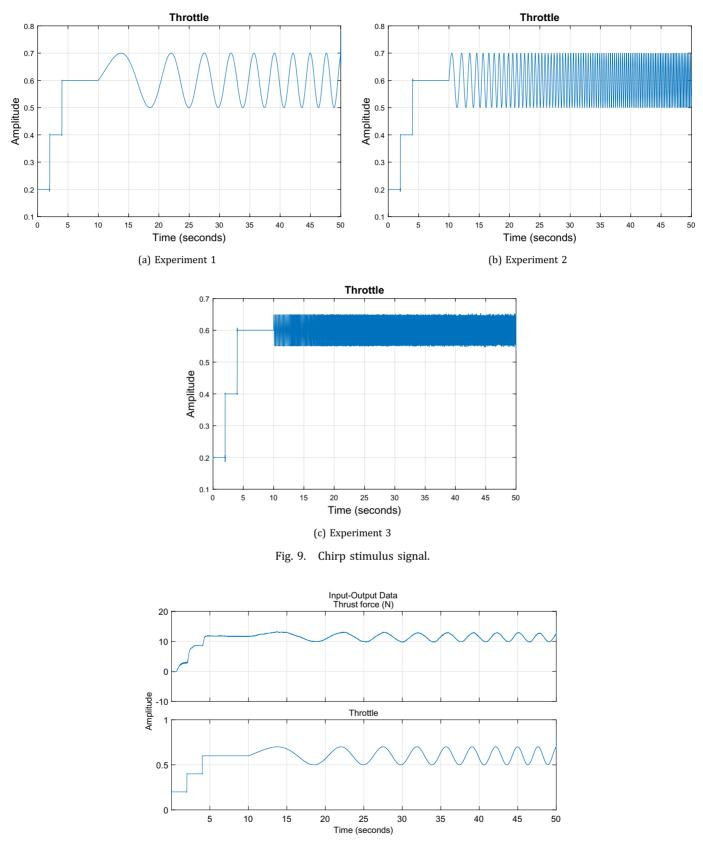
Fig. 10. Thrust channel, time domain data of experiment 1.
