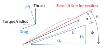
Fig. 3. Schematic of blade section aerodynamics.
