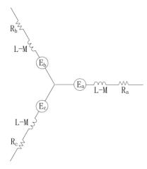
Fig. 2. General BLDC equivalent circuit.
