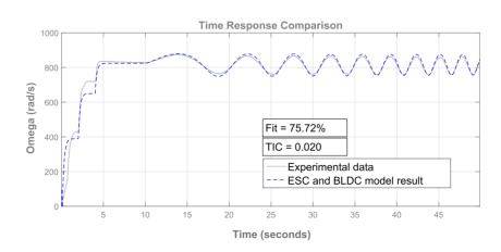
Fig. 17. Angular speed comparison between the semi-empirical MEP model prediction and experiment data (Experiment 1).
