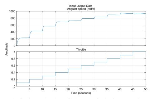
Fig. 8. Plot of measured angular speed with corresponding throttle in step signal test.
