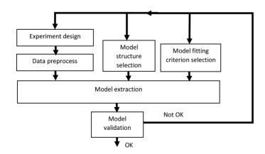
Fig. 1. System identification work flow.
