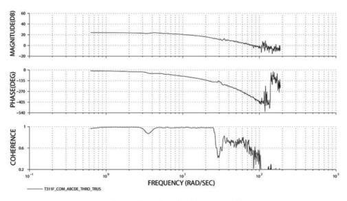
Fig. 13. Thrust channel, Bode plot estimated by CIFER.
