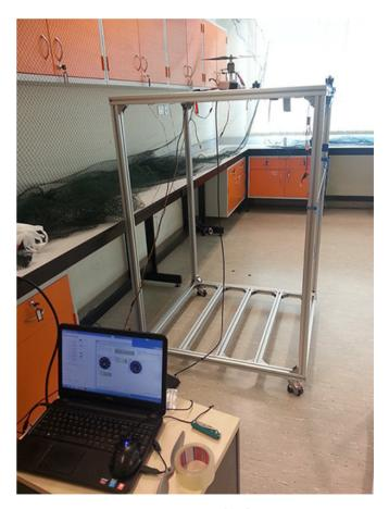
Fig. 6. Rotor experiment hardware setup.
