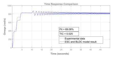
Fig. 18. Angular speed comparison between the semi-empirical MEP model prediction and experiment data (Experiment 2).
