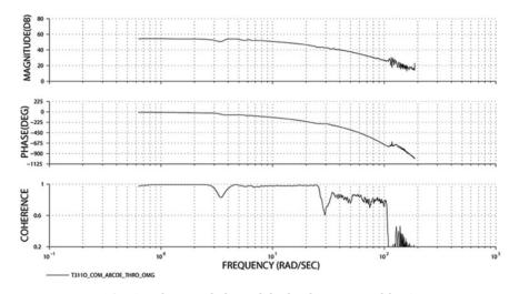
Fig. 15. Angular speed channel, bode plot estimated by CIFER.
