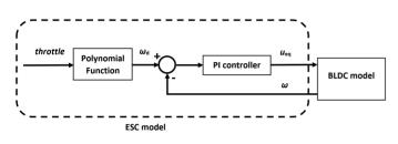
Fig. 4. Schematic of ESC model.
