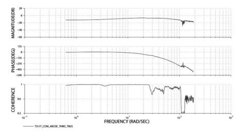
Fig. 14. Torque channel, Bode plot estimated by CIFER.
