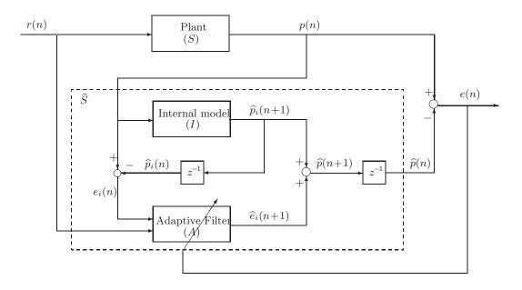
Figure 2 Block diagram of structure of the proposed system adaptation framework
