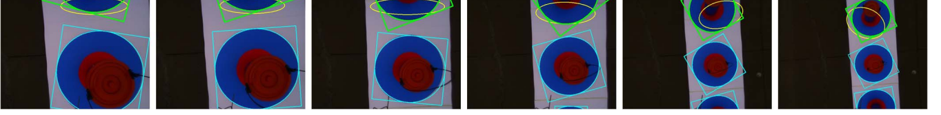
Fig. 8. Example to demonstrate ellipse tracking over consecutive images. The target ellipse is the top one (highlighted in green). The yellow ellipse is the target area returned by CAMShift.
