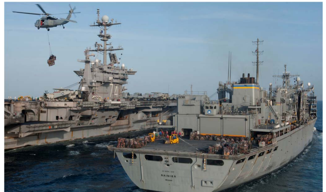
Fig. 2. Ship-to-ship vertical replenishment. (Use of released U.S. Navy imagery does not constitute product or organizational endorsement of any kind by the U.S. Navy.)
