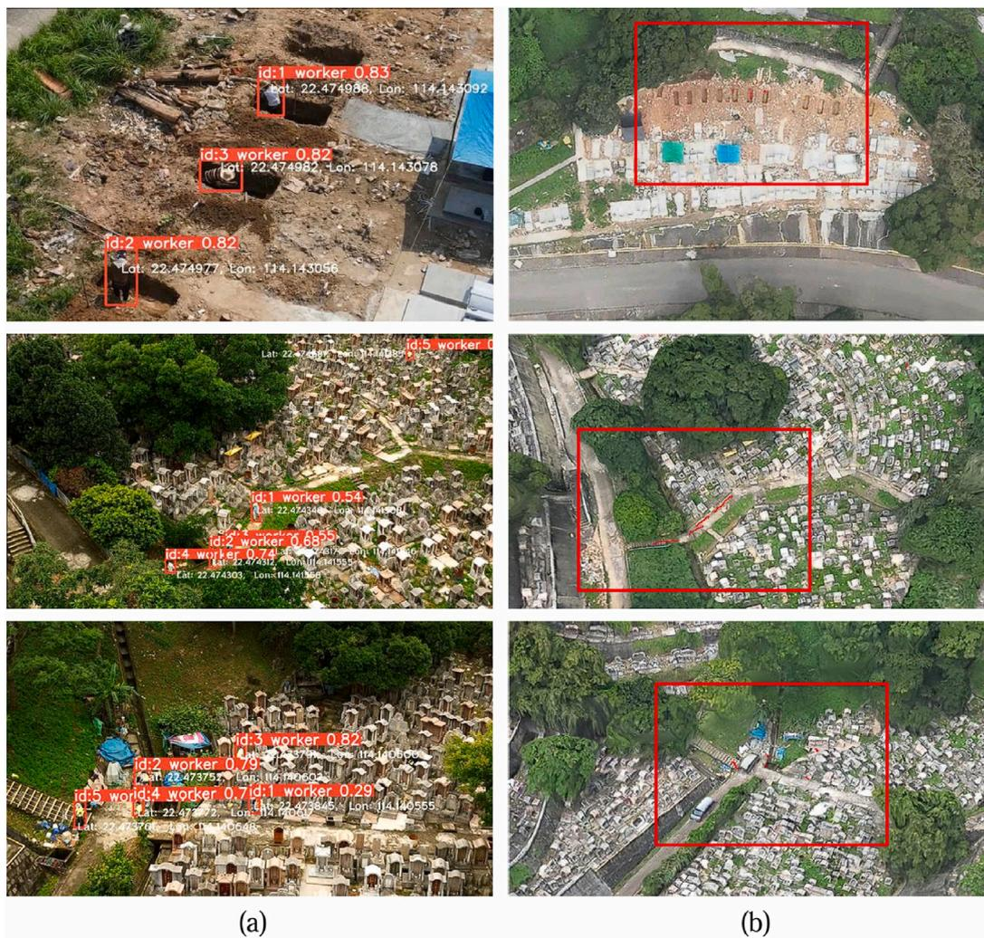
Fig. 17. (a) Real-time detection and tracking of workers with GPS information. (b) Historical trajectories of workers' localization on geo-referenced 3D model, with the red box indicating working region.
