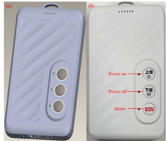
**Fig. 13.** (a) Design diagram of electronic work permit. (b) Physical representation of the electronic work permit.
