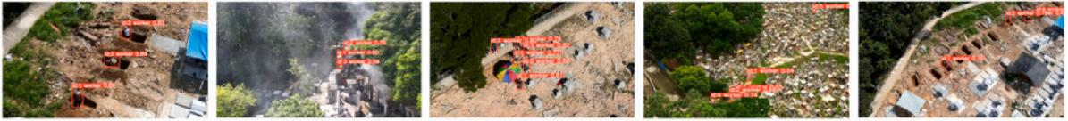
Fig. 12. Results of real-time worker detection and tracking.
