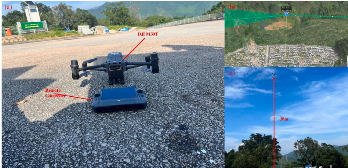
Fig. 10. (a) DJI M30T and its controller. (b) Sample inspection site with flight path in virtual space. (c) Drone following the designed flight path in physical space.
