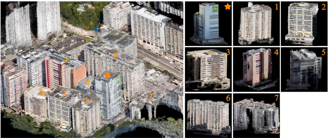
Fig. 6. The point cloud model of the target building and surrounding buildings reconstructed by LCM based MVSNet.
