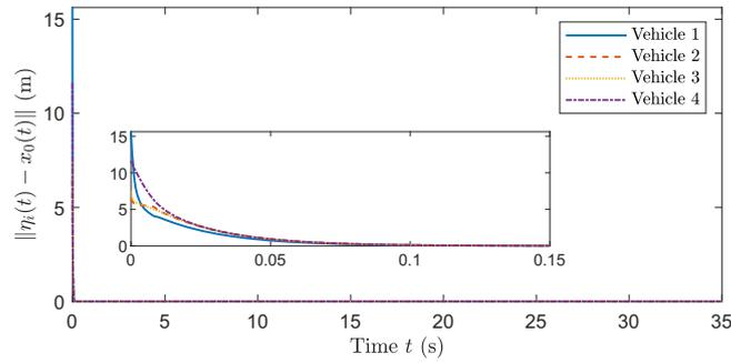
FIGURE 7 Estimation errors of the trajectory of the target.
