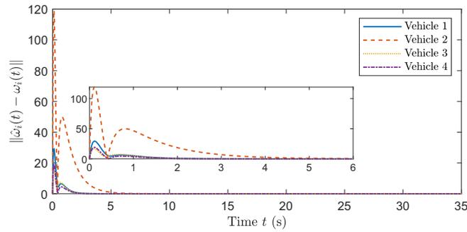
FIGURE 8 Estimation errors of the external disturbances.
