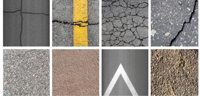
Fig. 1. The diverse appearances of roads with and without cracks. Row 1: Different types of cracks. Row 2: Various road backgrounds. Both cracks and background vary in appearance significantly, and may with much noise, dark shadow, and inconsistent brightness, etc.
