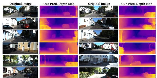
Fig. 7. Network prediction results of the depth estimation by trained models on the test set of KITTI Benchmark. Darker means deeper.
