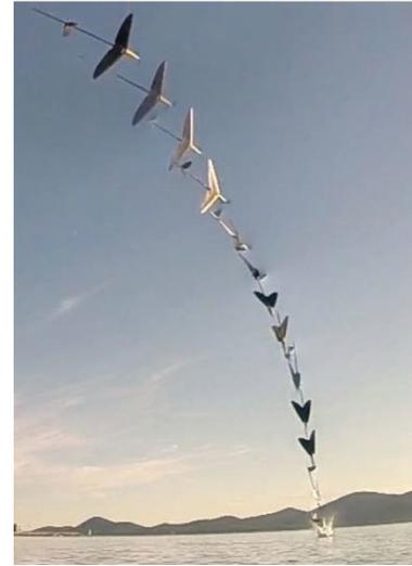
Fig. 4. The AquaMAV executing a plunge dive into the water. Image reproduced with permission from [24], courtesy of the authors and publishers.
