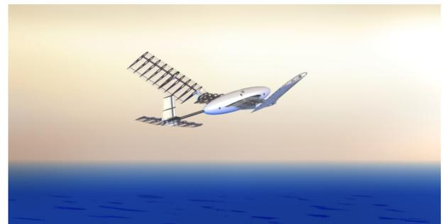
Fig. 13. The dual aerial/aquatic flapping vehicle concept from Massachusetts Institute of Technology. Image reproduced with permission from [55], courtesy of the authors and publishers.
