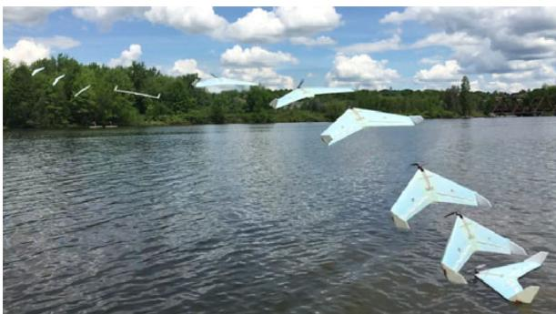
Fig. 1. The *SUWAVE* is a flying wing vehicle that uses water surfaces as resting areas to perform ‘lake-hopping’. Image reproduced with permission from [13], courtesy of the authors and publishers.
