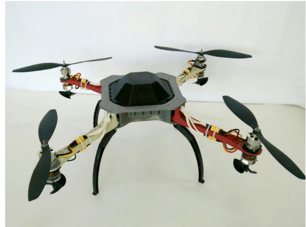
Fig. 10. A prototype of the HUAUV from Universidade Federal do Rio Grande. Image reproduced with permission from [49], courtesy of the authors and publishers.
