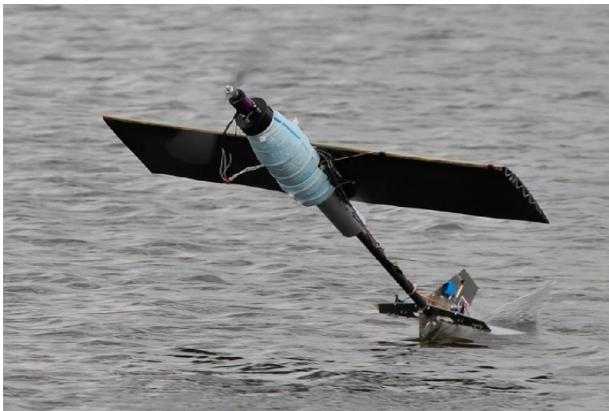
Fig. 6. The seabird-inspired fixed wing hybrid UAV-UUV by North Carolina State University and Teledyne. Image reproduced with permission from [30], courtesy of the authors and publishers.
