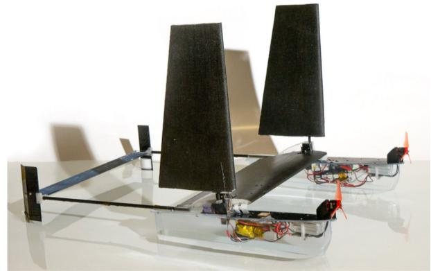
Fig. 2. The *SailMAV* is a fixed wing vehicle that can be converted into a sail boat configuration. Image reproduced with permission from [14], courtesy of the authors and publishers.
