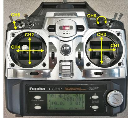
Fig. 4. Futaba 7CHP transmitter used for the prototype.
