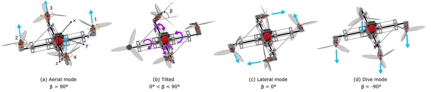
Fig. 3. Schematic diagram showing the axes convention and motor labeling used, as well as the different configurations possible with various values of the tilt angle  $\beta$ .
