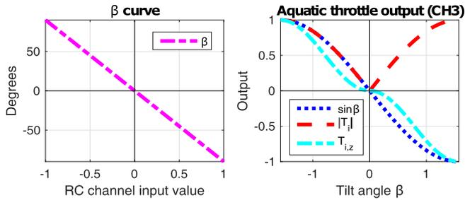
Fig. 7. Output curves associated with the mixed input CH3 that includes both the tilt angle  $\beta$  and thruster output.
