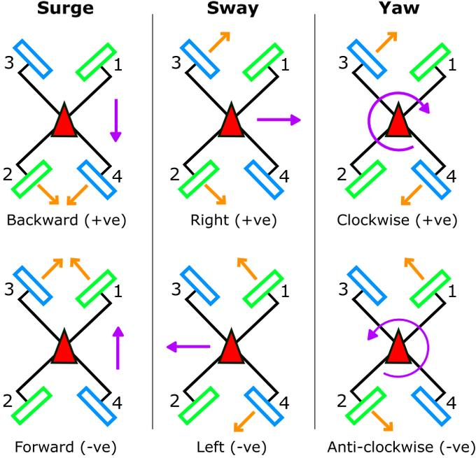
Fig. 5. Diagram showing the how inputs in lateral mode ( $\beta = 0$ ) corresponds to the planar movement of the vehicle. The direction (+ve/-ve) indicated refers to the direction of the input that will activate the motors shown.
