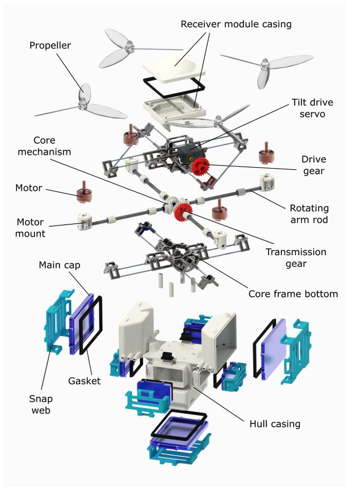
Fig. 2. Exploded rendering of the current prototype.
