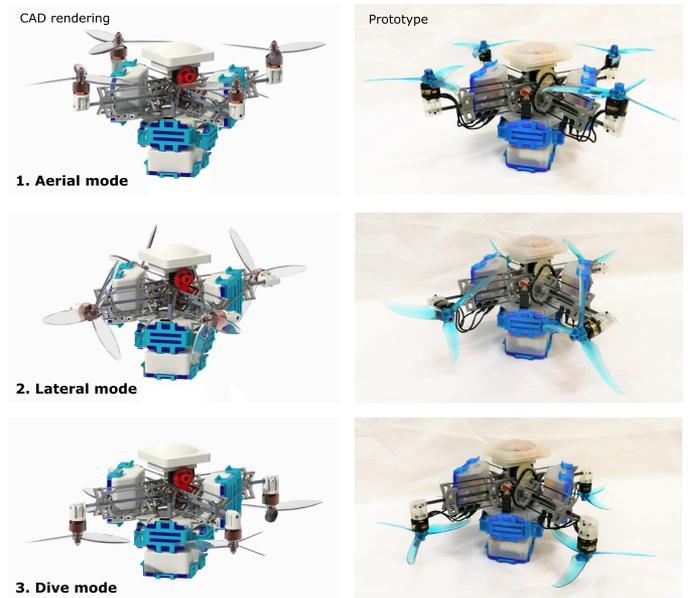
Fig. 1. CAD rendering (L) and the current prototype (R) of the proposed morphable aerial-aquatic quadrotor showing the rotors tilted at various angles and configurations.
