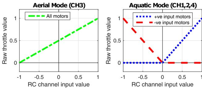
Fig. 6. Throttle curves for the aerial and aquatic modes differ in both the motors actuated and output mapping.
