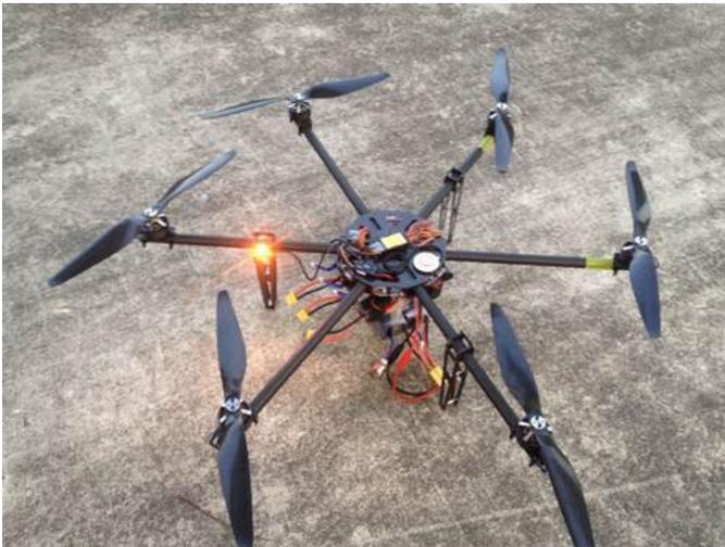
Fig. 15. A customized hexrotor platform.
