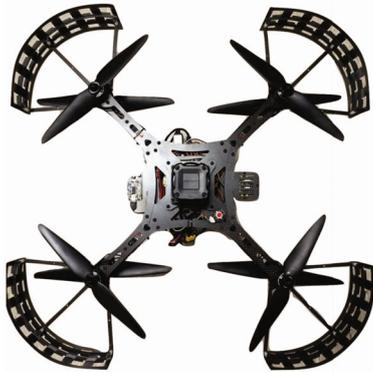
Fig. 10 The X8 configuration octocopter BL-068 from ALT.
