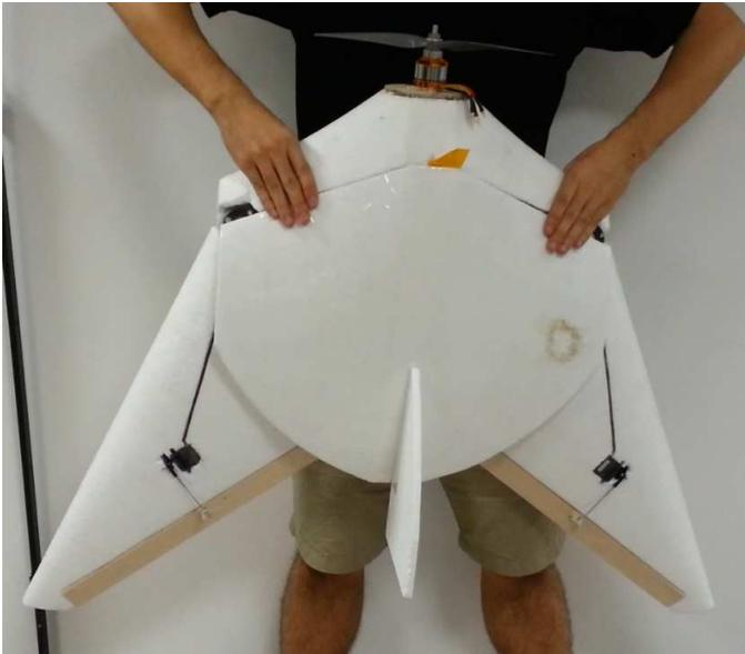
Fig. 24. U-Lion Mark II (without tail) with wings folded.
