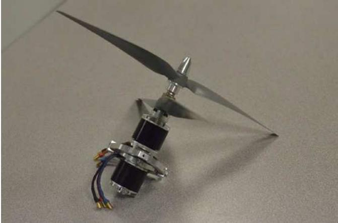
Fig. 29. The self-customized contra-rotating motor.
