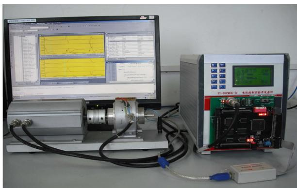
**Fig. 4.** Experimental setup of PMSM servo system.
