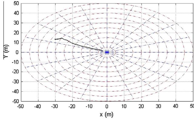
Fig. 22. The distance of the follower from the desired position in Scenario 3.
