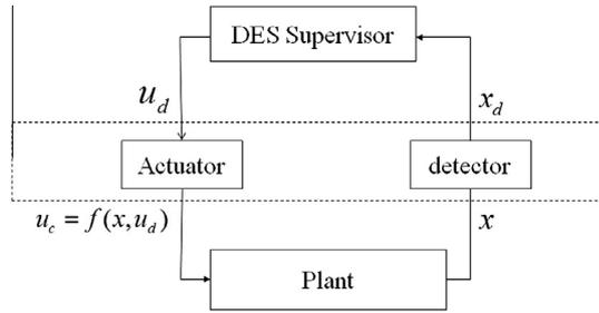
Fig. 4. Linking the discrete supervisor to the plant via an interface layer.
