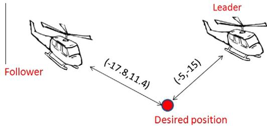
Fig. 11. The schematic of the scenario with for a leader–follower case tracking a line (Scenario 2).
