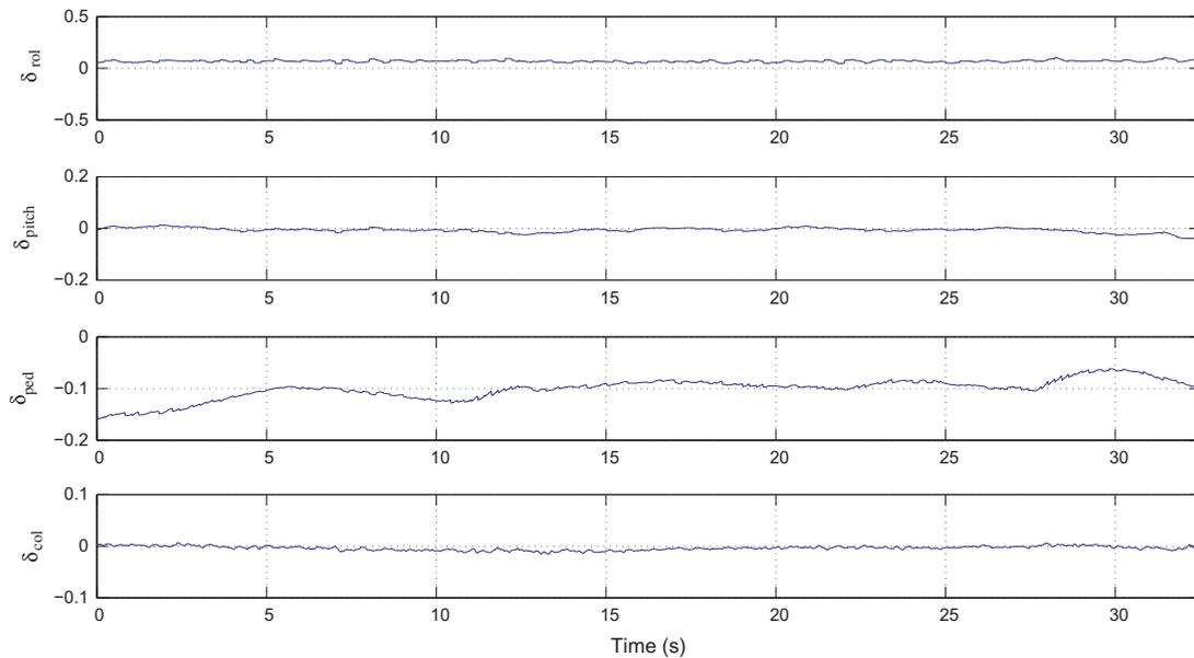
Fig. 9. Control signals of the follower UAV in Scenario 1.
