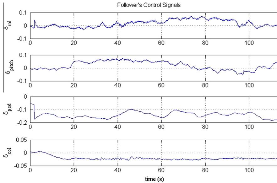
Fig. 20. Control signals of the follower UAV in Scenario 3.
