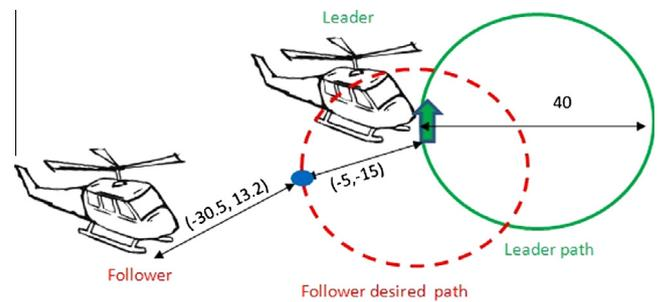
Fig. 17. The schematic of the scenario with for a leader–follower case tracking a circle (Scenario 3).
