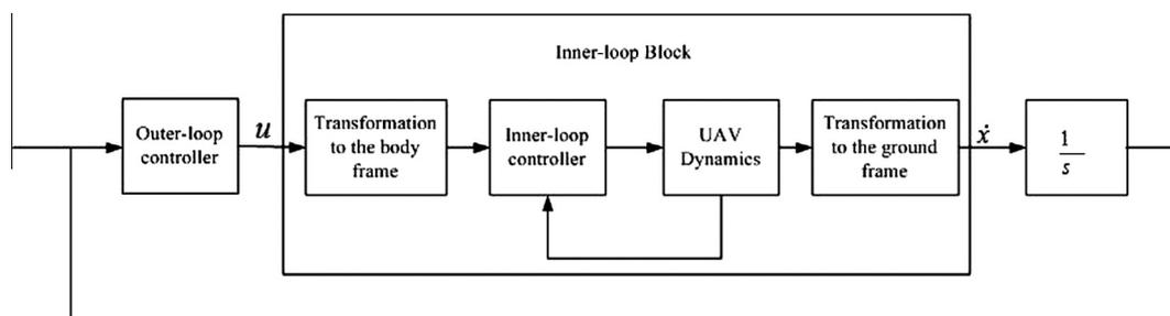
Fig. 2. The control structure of the NUS UAVs.
