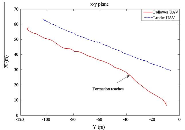
Fig. 12. The position of the UAVs in the x–y plane in Scenario 2.
