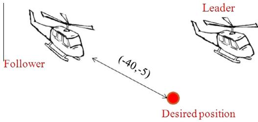
Fig. 7. The schematic of the scenario with a real follower and a virtual fixed leader (Scenario 1).
