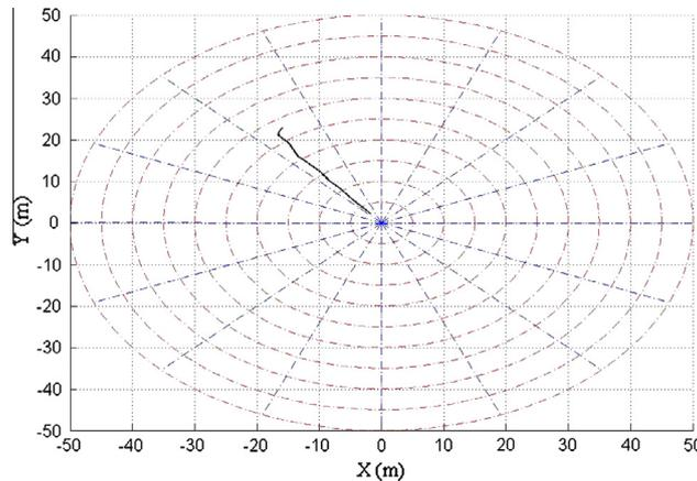
Fig. 24. The relative distance between the UAVs projected onto x-y plane in Scenario 3.
