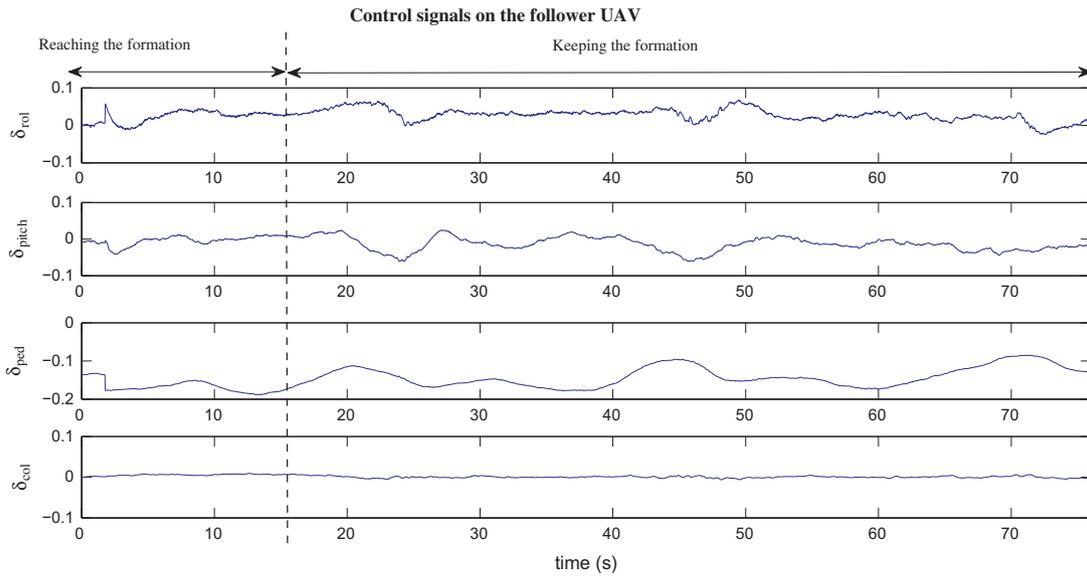
Fig. 14. Control signals of the follower UAV in Scenario 2.
