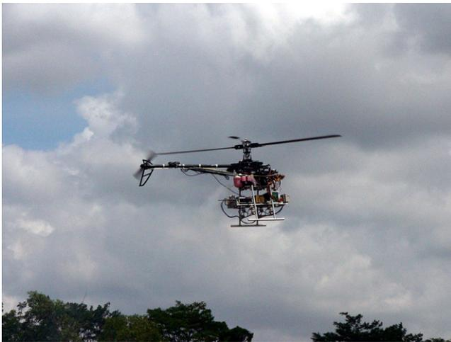
Fig. 2. HeLion—a fully autonomous unmanned helicopter.
