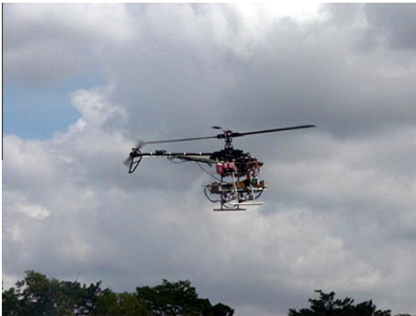
Fig. 1. HeLion, a small-scale UAV helicopter.
