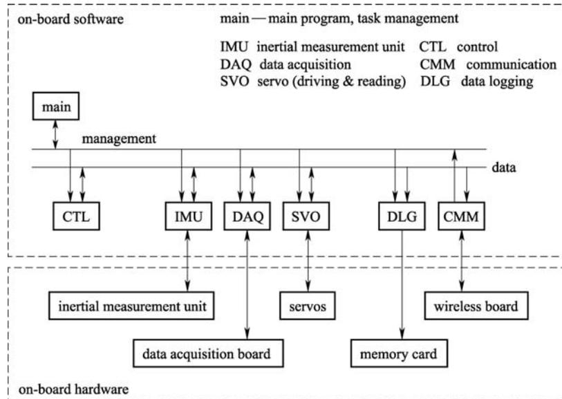
Fig. 8 Framework of an avionic software system
