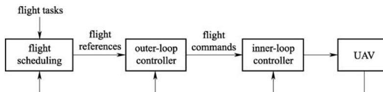
Fig. 10 Structure of overall autonomous flight control
