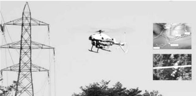
Fig. 14 Sky Surveyor inspecting power transmission line
