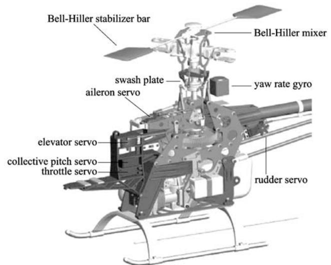
Fig. 3 Typical hardware configuration of single-rotor RC helicopter
