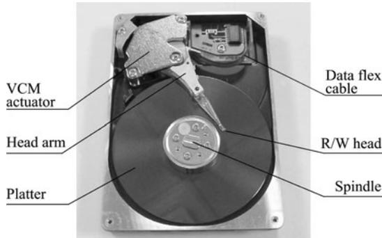
Fig. 7 A typical HDD with a VCM actuator.
