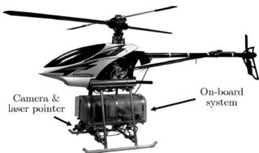
Figure 2 SheLion: a vision-capable unmanned helicopter.
