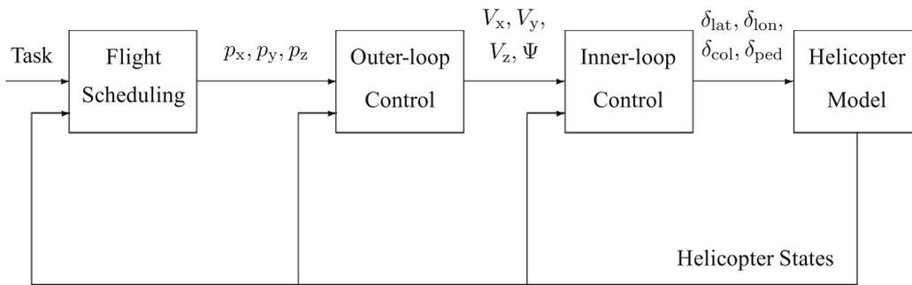
Fig. 4. Automatic flight control structure of the UAV helicopter system.
