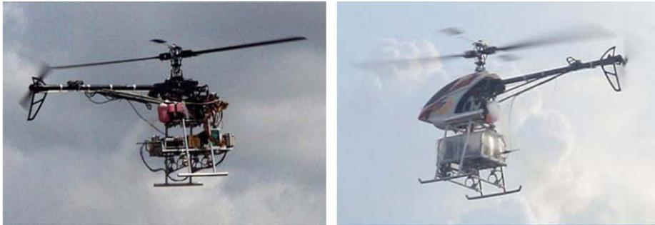
Fig. 1. The UAV helicopters, HeLion and SheLion.
