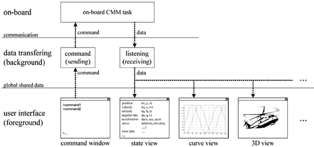
Fig. 8. The structure of the ground station software system.
