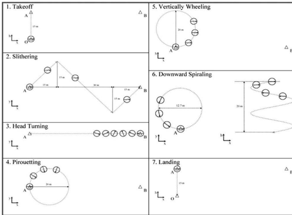
Fig. 12. Flight schedule of the full-envelope flight test.
