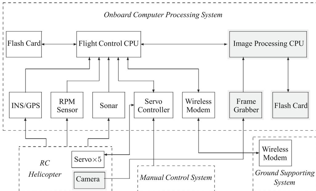
Fig. 3. Hardware configuration of the UAV helicopter system, SheLion.
