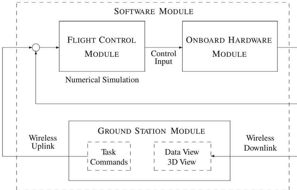
Fig. 2. Framework of the hardware-in-the-loop simulation of the UAV system.
