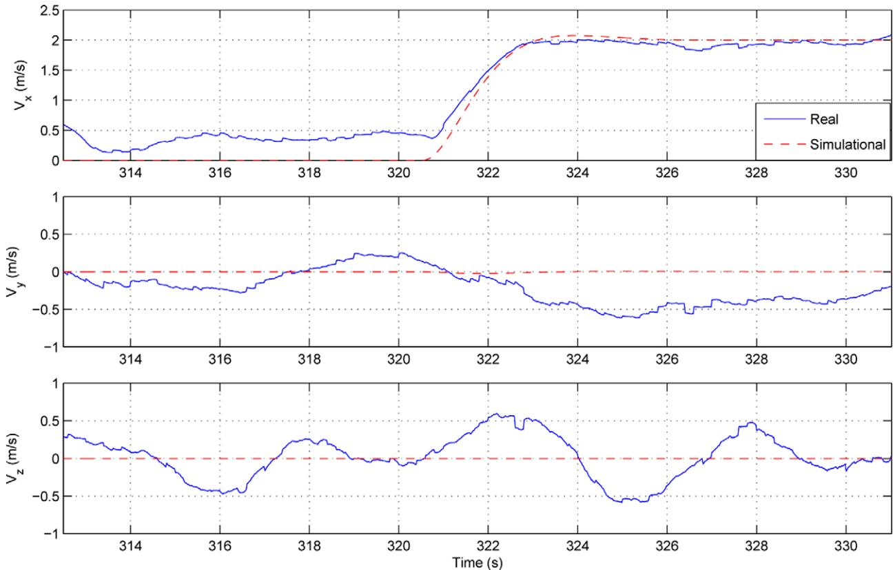
Fig. 9. Velocities of hardware-in-the-loop simulation and actual flight tests.
