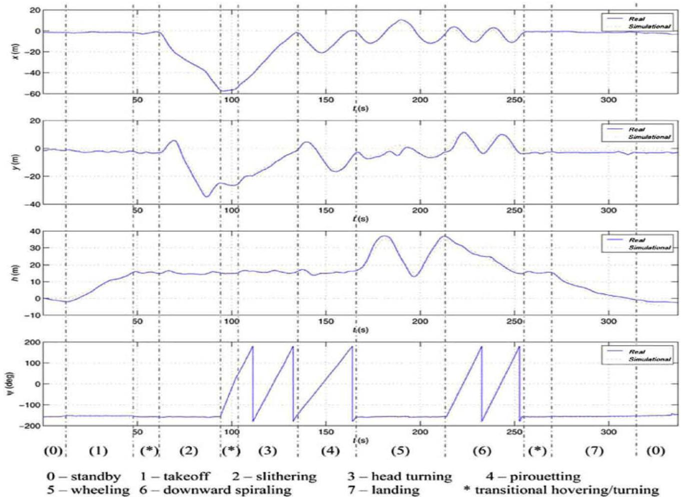
Fig. 13. Results of hardware-in-the-loop simulation and real flight test for full-envelope flight case.
