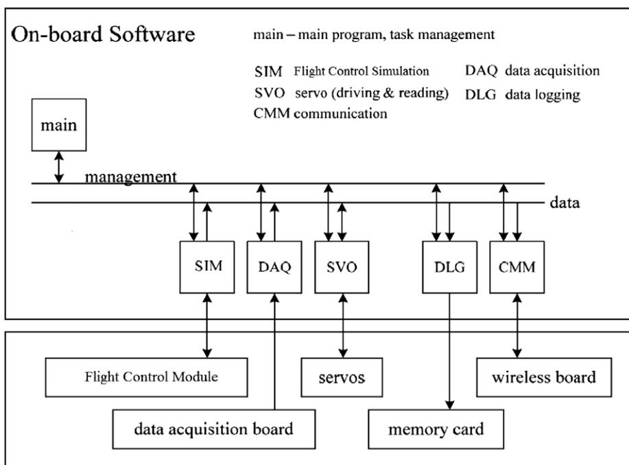
Fig. 7. The structure of the onboard software system.
