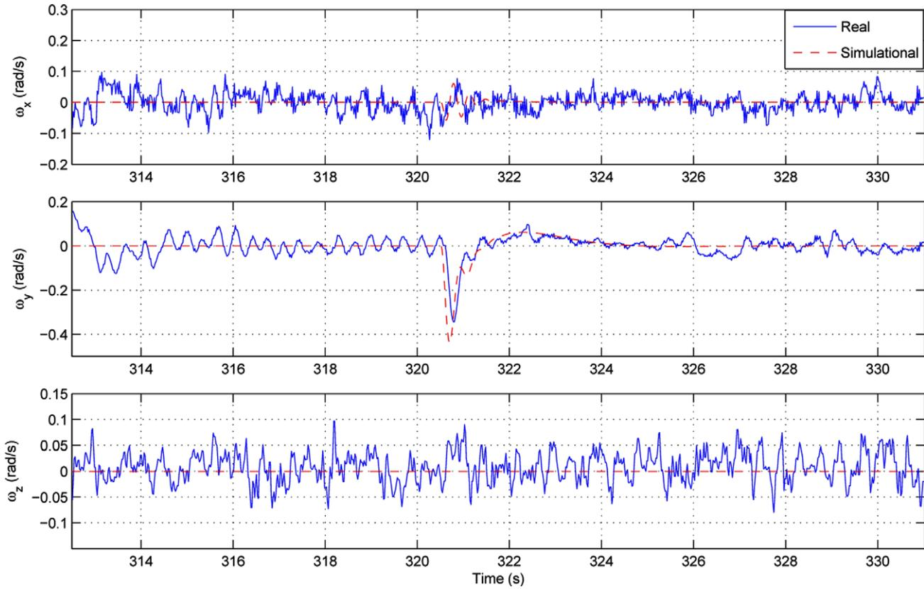
Fig. 10. Angular rates of hardware-in-the-loop simulation and actual flight tests.
