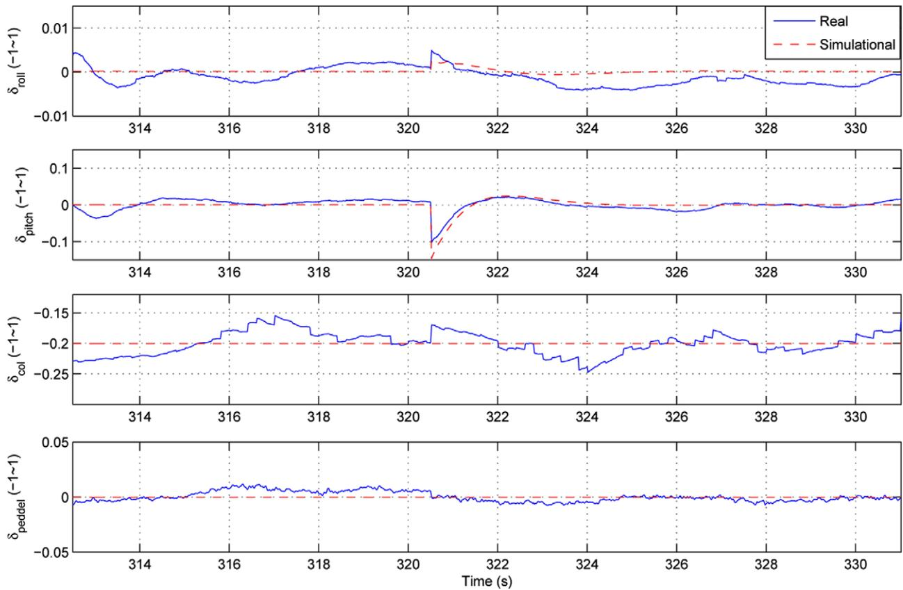
Fig. 11. Input signals of hardware-in-the-loop simulation and actual flight tests.
