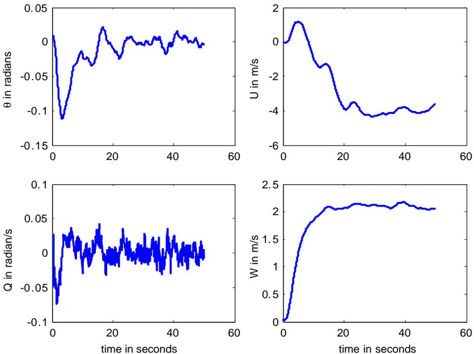
**Fig. 10** Closed-loop longitudinal state responses to a unity bank angle step demand
