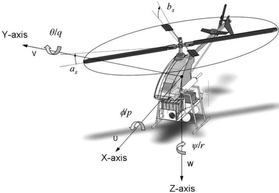
**Fig. 3** Helicopter states in body frame coordinate system
