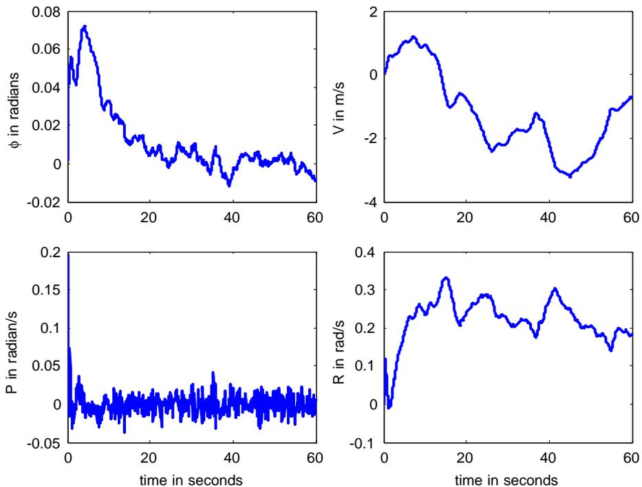
**Fig. 13** Closed-loop lateral-directional state responses to a unity pitch angle step demand
