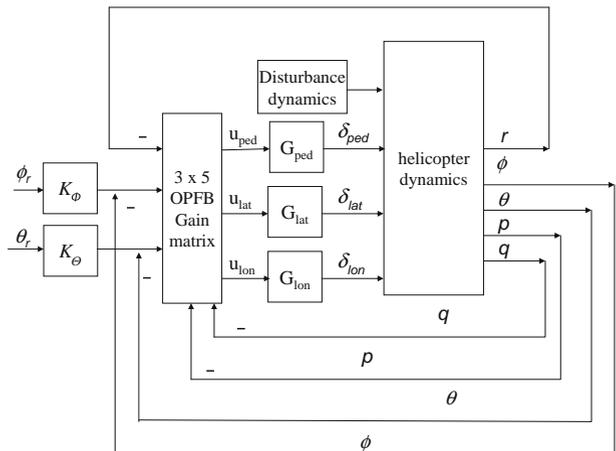
**Fig. 5** Loop shaped plant with controller
