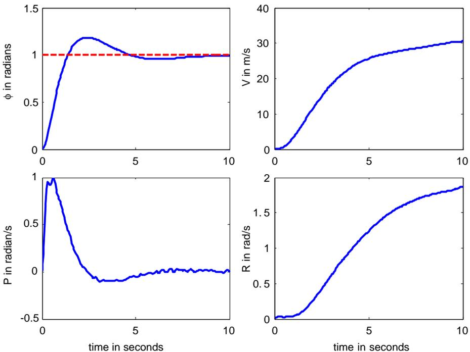
**Fig. 9** Closed-loop lateral-directional state responses to a unity bank angle step demand
