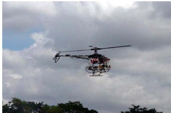
Fig. 1. UAV helicopter, HeLion.
