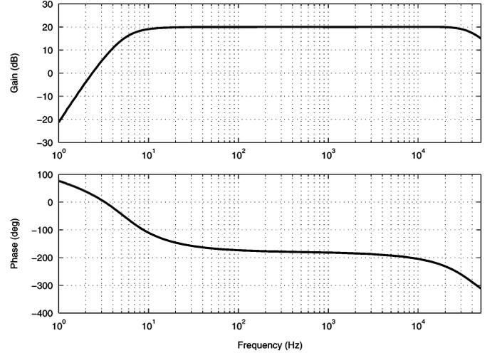
Fig. 4. Frequency response of differential amplifier setup consisting of HP1142A differential probe control and Brüel and Kjær voltage amplifier.
