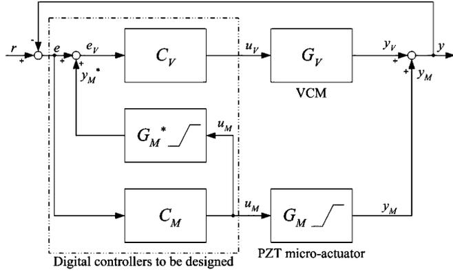
Fig. 1. Modified DMS configuration with PZT microactuator saturation considerations [4].
