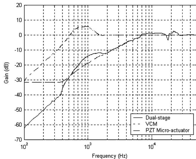
Fig. 20. Experimental sensitivity transfer functions using proposed SSA-DMS dual-stage control topology.
