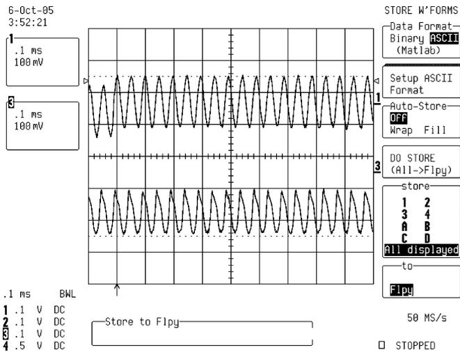
Fig. 7. Time responses with  $u_M = 10 \sin(2\pi 30 \times 10^3 t)$  V. (Top) PZT microactuator's displacement  $y_M$  measured from LDV with resolution of  $0.5 \mu\text{m}/\text{V}$ . (Bottom) Estimated PZT microactuator's displacement  $y_M^*$  from digital bridge circuit inverse  $H_B^{-1}(z)$ . The PZT microactuator is actuating at about  $\pm 37.5$  nm in radial directions.
