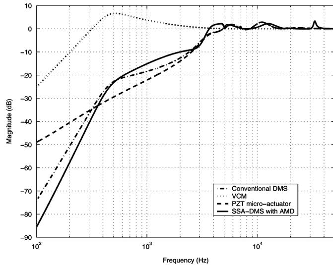
Fig. 19. Simulated sensitivity transfer functions of different control schemes.
