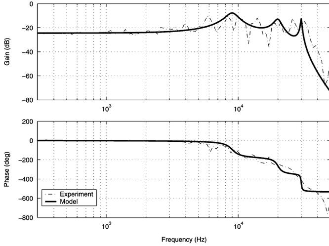
Fig. 5. Frequency response of displacement estimation circuit  $H_B$ .TABLE I
