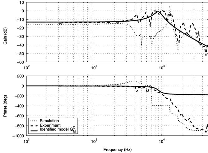
Fig. 15. Identified model of PZT microactuator with AMD control.
