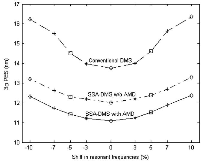
Fig. 21. Comparison of  $3\sigma$  PES with different control schemes.
