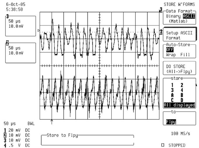
Fig. 9. Time responses with  $u_M = 1.2 \sin(2\pi 30 \times 10^3 t)$  V. (Top) PZT microactuator's displacement  $y_M$  measured from LDV with resolution of  $0.5 \mu\text{m}/\text{V}$ . (Bottom) Estimated PZT microactuator's displacement  $y_M^*$  from digital bridge circuit inverse  $H_B^{-1}(z)$ . The PZT microactuator is actuating at about  $\pm 5$  nm in radial directions.
