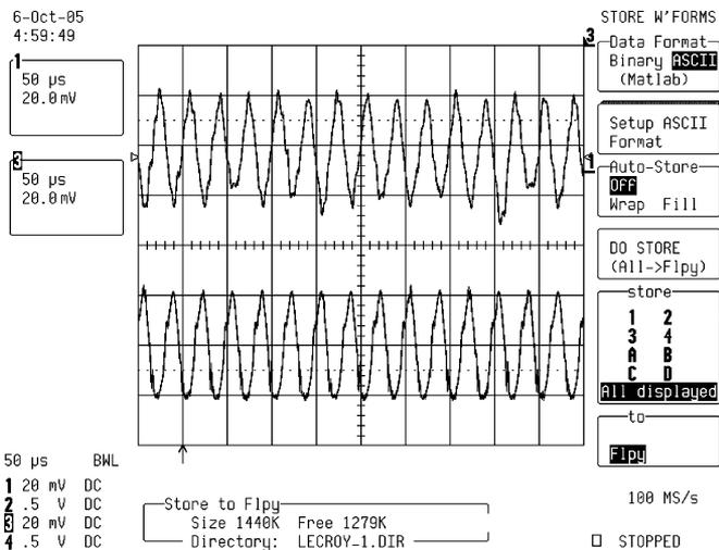
Fig. 8. Time responses with  $u_M = 2.5 \sin(2\pi 30 \times 10^3 t)$  V. (Top) PZT microactuator's displacement  $y_M$  measured from LDV with resolution of  $0.5 \mu\text{m}/\text{V}$ . (Bottom) Estimated PZT microactuator's displacement  $y_M^*$  from digital bridge circuit inverse  $H_B^{-1}(z)$ . The PZT microactuator is actuating at about  $\pm 10$  nm in radial directions.
