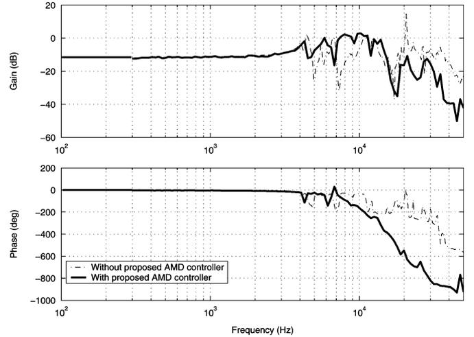
Fig. 13. Experimental frequency responses of PZT microactuator.
