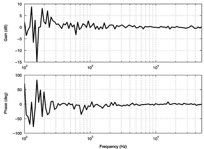
Fig. 10. Frequency response of measured PZT microactuator's displacement from LDV  $y_M$  to estimated PZT microactuator's displacement  $y_M^*$ . The PZT microactuator is set to actuate at about  $\pm 8$  nm in radial directions.
