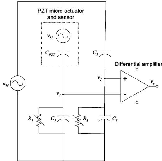
Fig. 3. Bridge circuit employing the PZT microactuator as actuator and sensor simultaneously. The PZT elements are modeled as a capacitor  $C_{PZT}$  with dependent voltage  $v_M$ .
