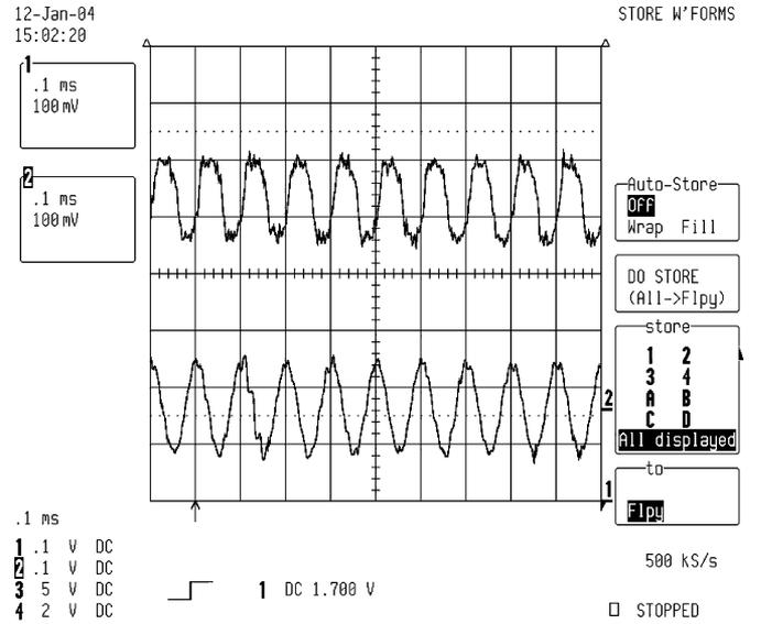
Fig. 6. Time responses with  $u_M = 10 \sin(2\pi 10 \times 10^3 t)$  V. (Top) PZT microactuator's displacement  $y_M$  measured from LDV with resolution of  $0.5 \mu\text{m/V}$ . (Bottom) Estimated PZT microactuator's displacement  $y_M^*$  from digital bridge circuit inverse  $H_B^{-1}(z)$ . The PZT microactuator is actuating at about  $\pm 37.5$  nm in radial directions.
