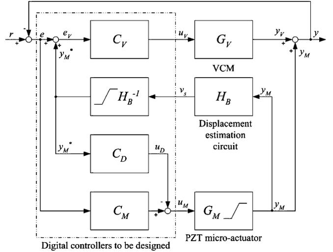
Fig. 2. Proposed SSA-DMS dual-stage control topology. The PZT microactuator's displacement estimation circuit  $H_B$  allows an online estimation of PZT microactuator's displacement  $y_M^*$ .
