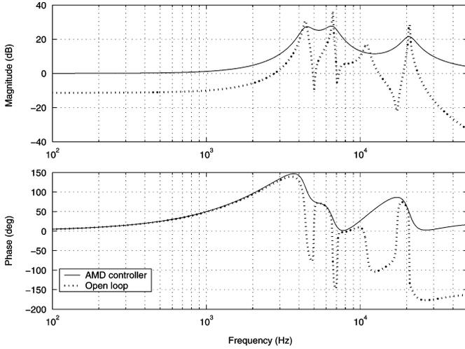
Fig. 12. Simulated frequency responses of PZT microactuator with AMD.
