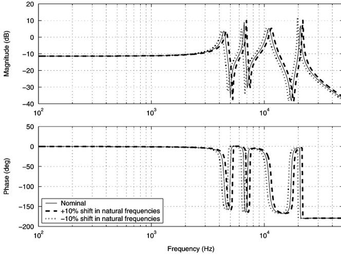
Fig. 16. Frequency responses of PZT microactuator with  $\pm 10\%$  shift in natural frequencies.
