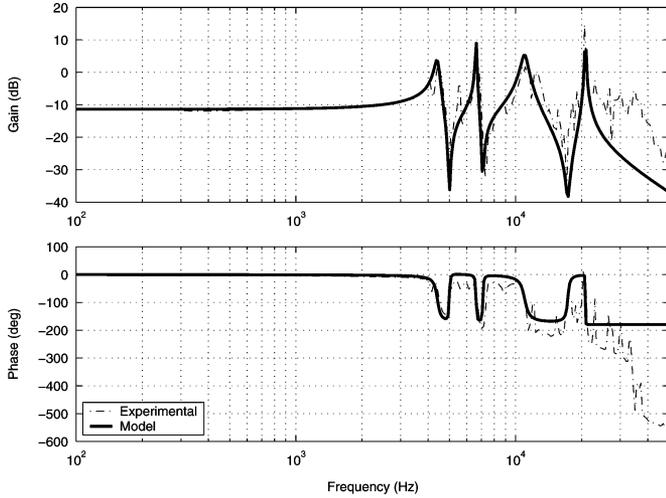
Fig. 11. Frequency response of PZT microactuator.
