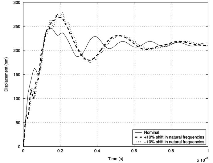
Fig. 18. Simulated step responses of PZT microactuator with  $\pm 10\%$ .
