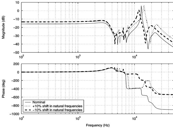
Fig. 17. PZT microactuator's inner closed-loop transfer functions.
