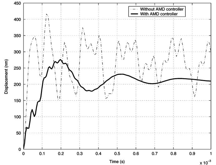
Fig. 14. Simulated step responses of PZT microactuator with and without AMD.
