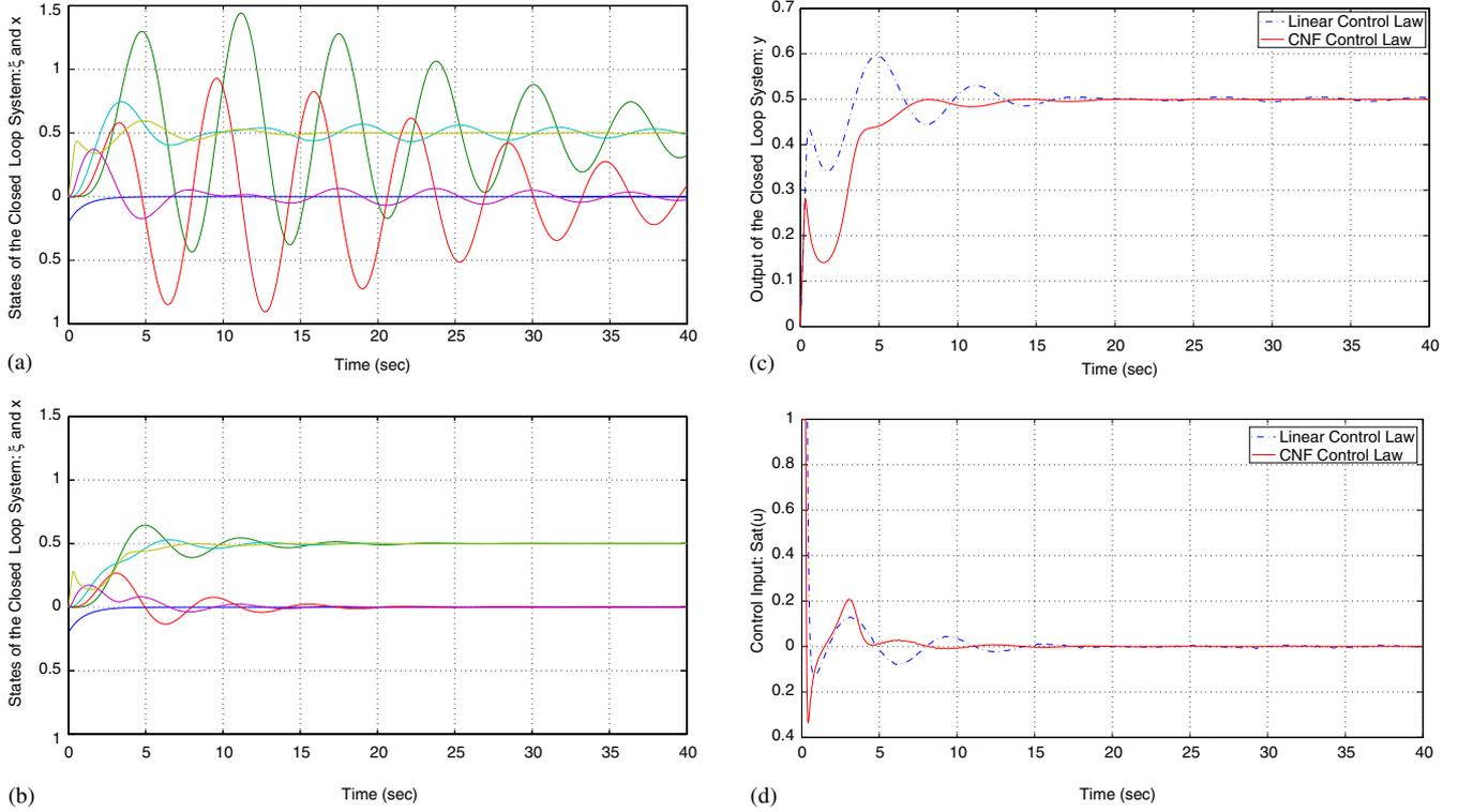
Fig. 2. State responses and control signals of the closed-loop systems. (a) State responses with the linear control law. (b) State responses with the CNF control law. (c) System output of the closed-loop system. (d) Control signals.
