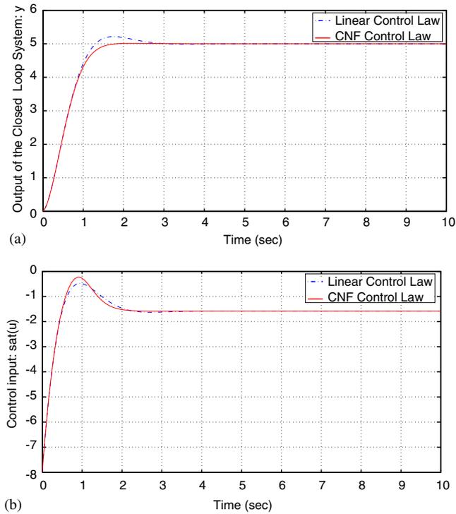
Fig. 3. Output responses and control signals of the flight control system. (a) Output responses. (b) Control signals.
