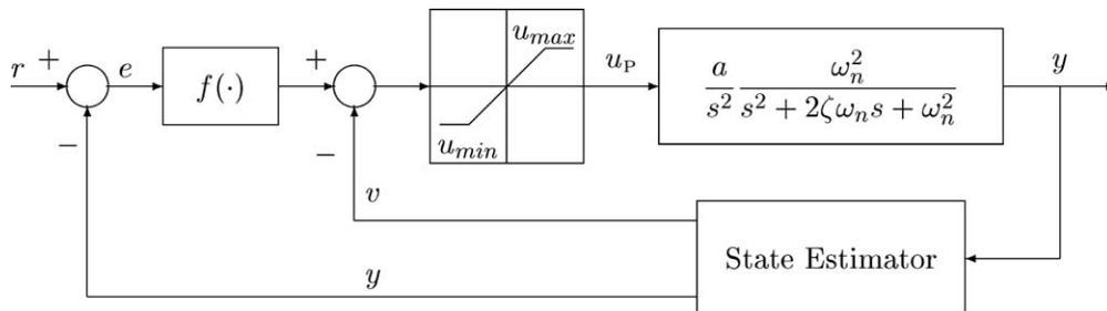
Fig. 4. The track seeking controller.
