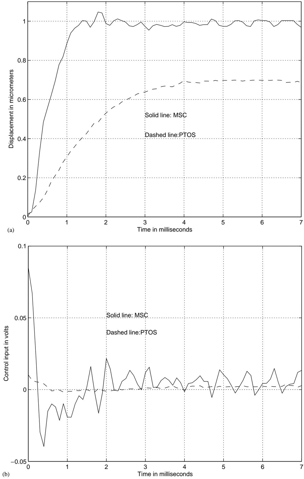
Fig. 7. Implementation results: response and control for 1  $\mu\text{m}$  displacement: (a) Output responses; (b) control signals.
