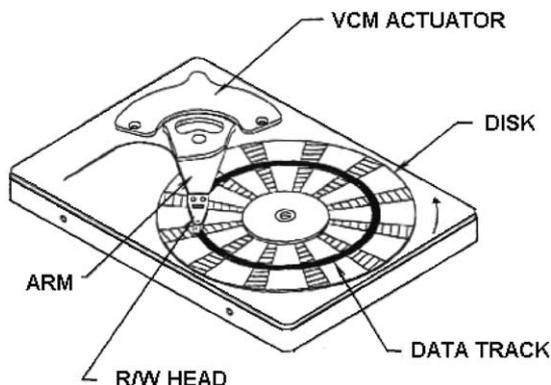
Fig. 1. A hard disk drive with a VCM actuator servo system.
