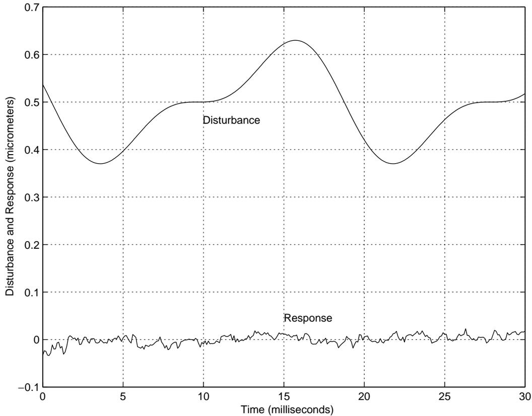
Fig. 9. Implementation result: response to a runout disturbance (MSC).
