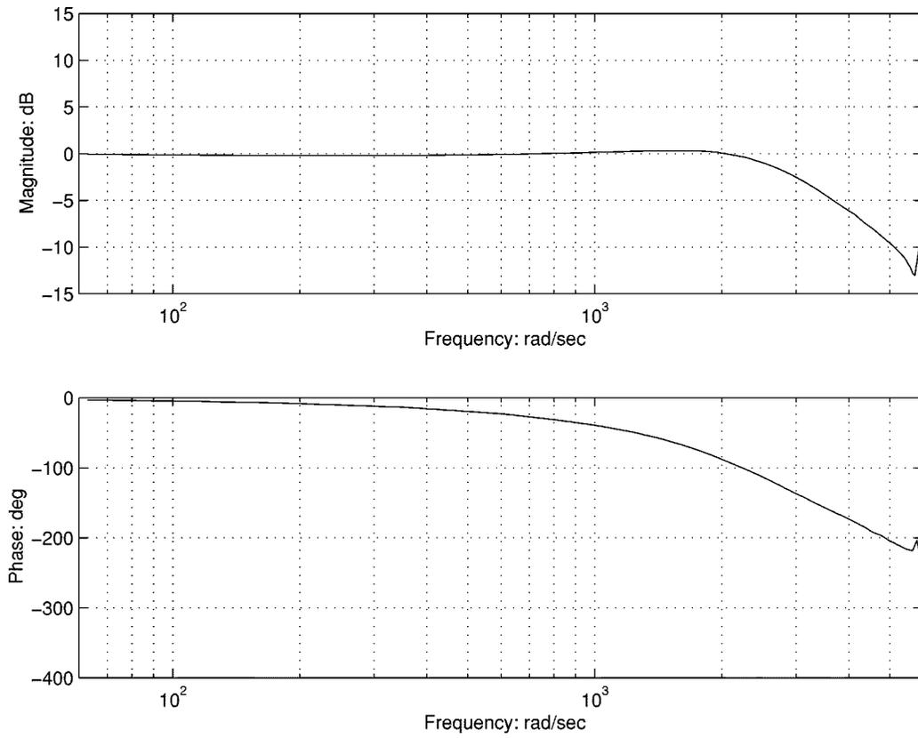
Fig. 8. Implementation result: Closed-loop frequency response of system with RPT controller.
