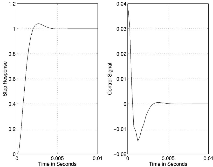
Fig. 4. Step response of the closed-loop system with the discretized RPT controller.
