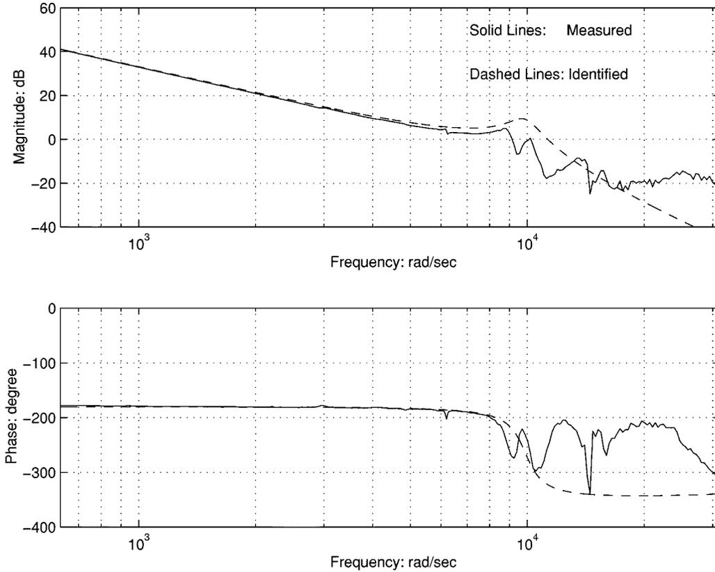
Fig. 2. Frequency responses of the actual and identified models of the VCM actuator.
