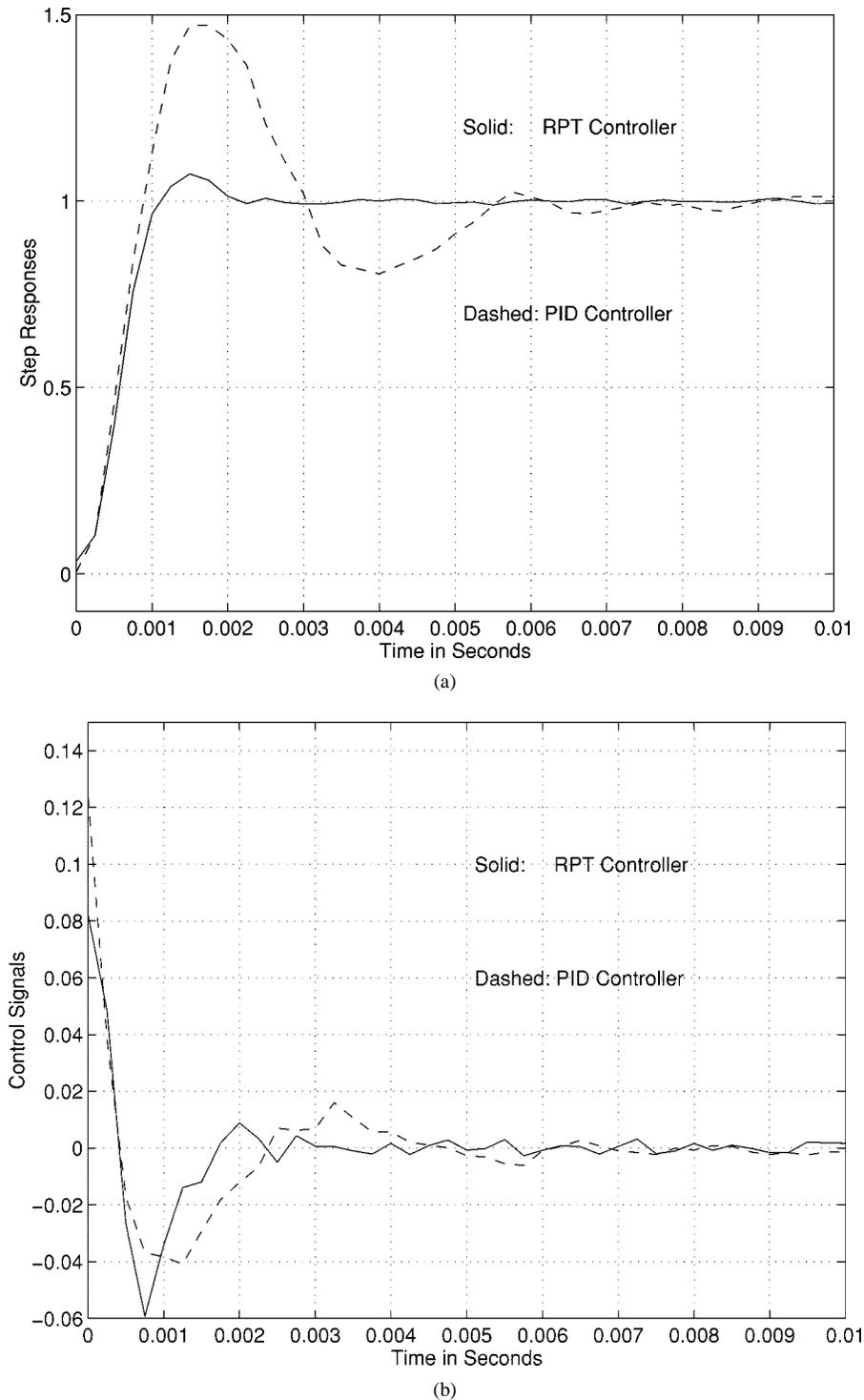
Fig. 7. Implementation result: Step responses of closed-loop systems with RPT and PID controllers.
