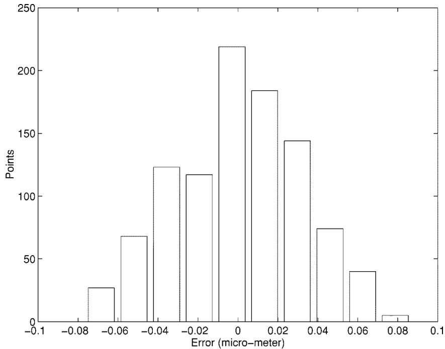
Fig. 10. Implementation result: Histogram of the PES test with the RPT controller.
