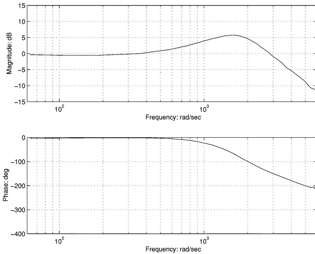
Fig. 9. Implementation result: Closed-loop frequency response of system with PID controller.
