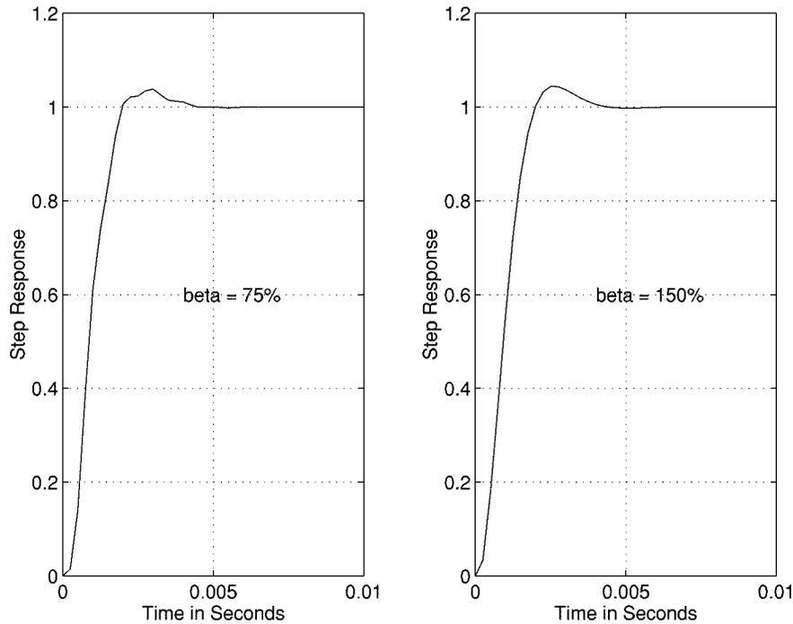
Fig. 5. Step responses of the closed-loop system with different resonant frequencies.
