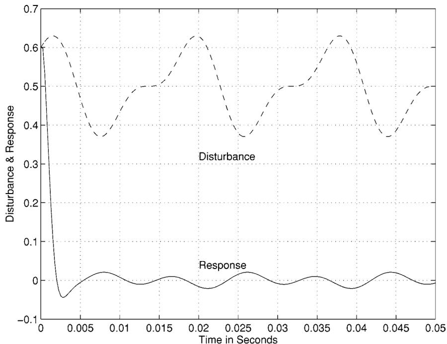
Fig. 6. Output response of the closed-loop system due to a run-out disturbance.
