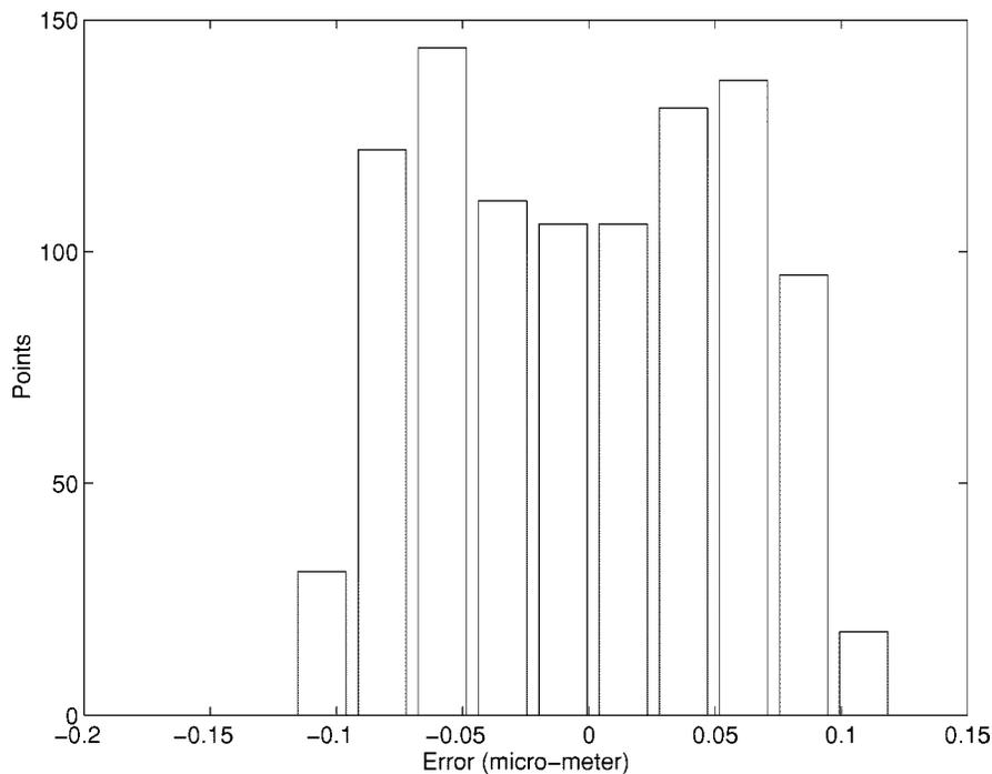
Fig. 11. Implementation result: Histogram of the PES test with the PID controller.
