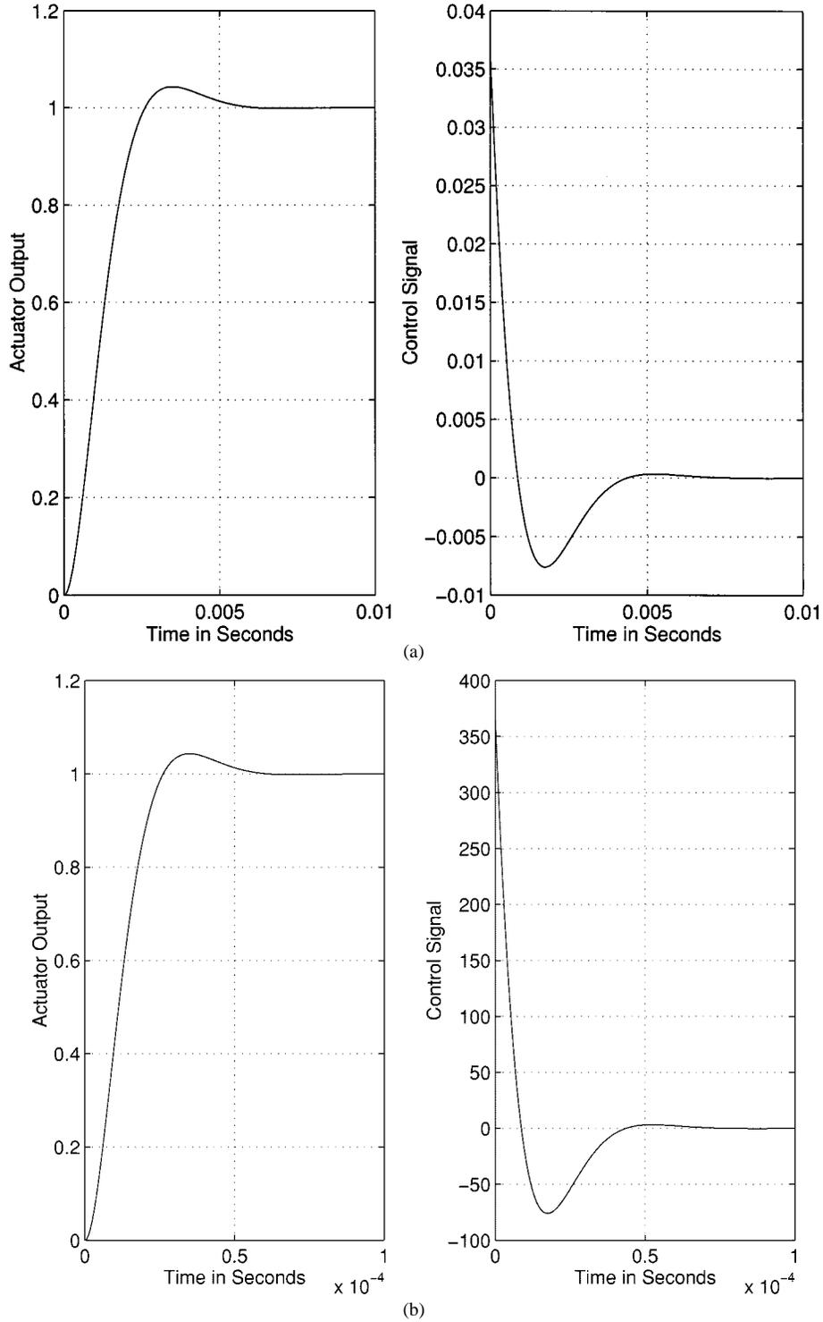
Fig. 3. Responses of the closed-loop systems with parameterized RPT controller. (a)  $\varepsilon = 1$ . (b)  $\varepsilon = 0.01$ .
