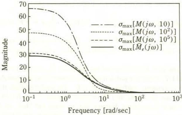
Fig. 4.2. Maximum singular values of  $\bar{M}^\epsilon(j\omega)$  and  $M(j\omega, \sigma)$ .
