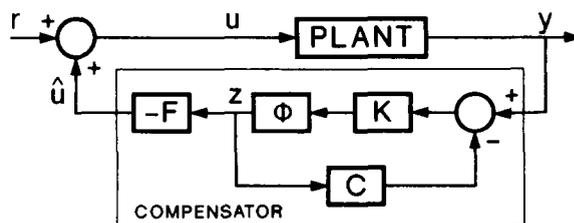
FIG. 3. Plant with full order compensator.
