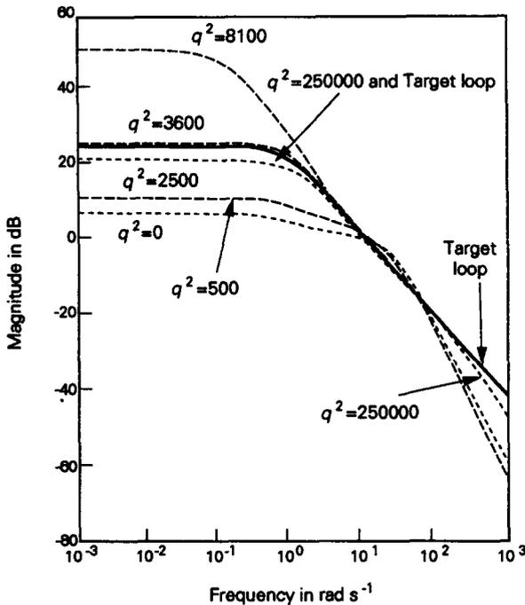
FIG. 6(a). Singular values of target loop and design loops.
