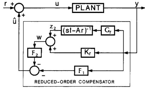
FIG. 5. Plant with reduced order compensator.
