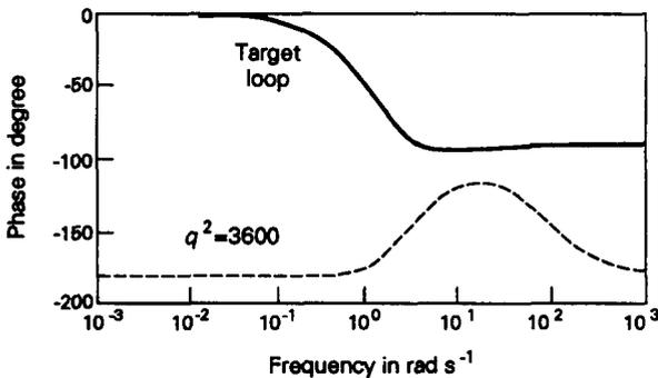
FIG. 6(b). Phase responses of target loop and design loop with  $q^2 = 3600$ .
