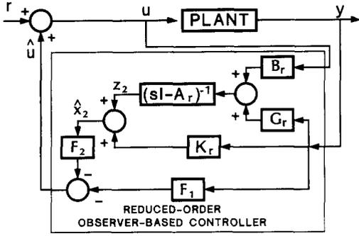
FIG. 4. Plant with reduced order observer based controller.
