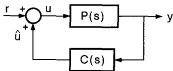
FIG. 1. Plant-controller closed-loop configuration.
