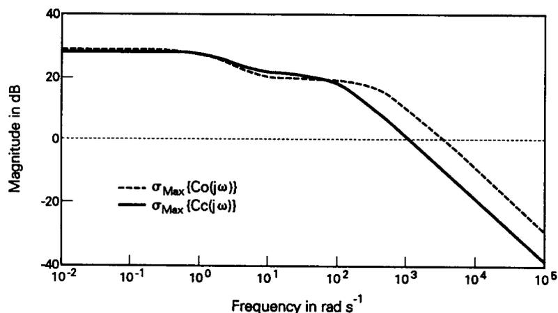
FIG. 7(b). Maximum singular values of full order observer based controller and compensator given in Table 1(b).
