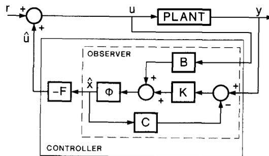
FIG. 2. Plant with full orders observer based controller.
