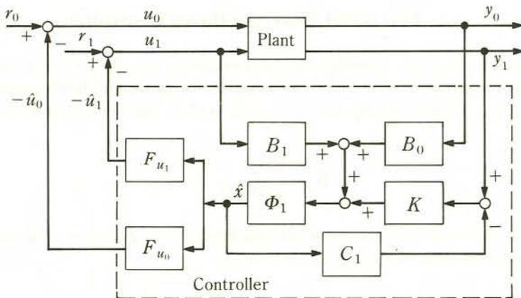
Fig. 2. Plant with the full order observer based controller.
