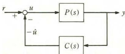
Fig. 1. Closed-loop configuration—plant with controller.
