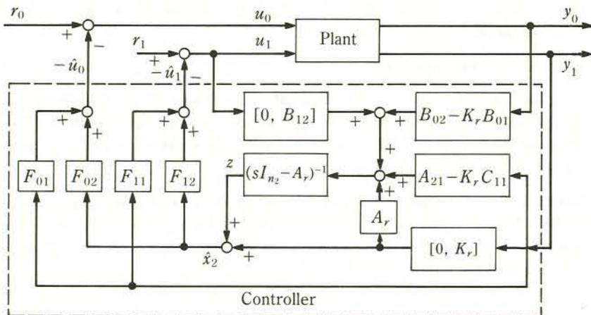
Fig. 3. Plant with the reduced order observer based controller.
