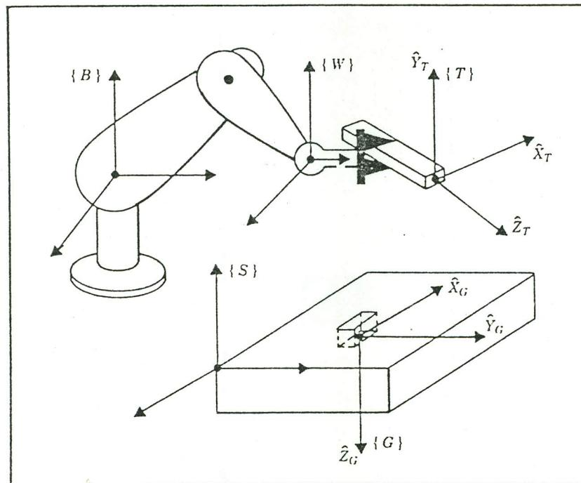
4. For the 2-link manipulator shown below, the link transformation matrices,  ${}^0 T_1$  and  ${}^1 T_2$ , were determined. Their product is:
