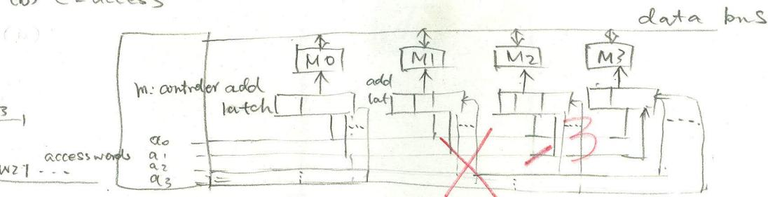
Address put in addr. latch, then adjust the access distance, we can have different sequential of data
