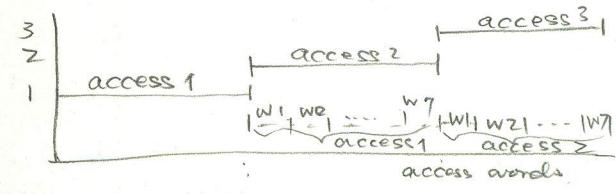
When the memory do accessing, all the modules access simultaneously to the latches and then multiplex select the word.
