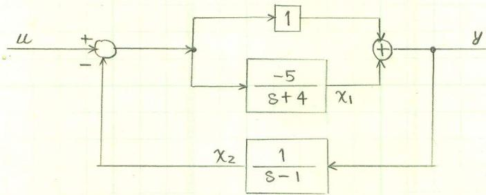
SOLUTION: Use some replacements. It will ~~make us~~ much easier to write the state equations. So, redraw the block diagram as:
