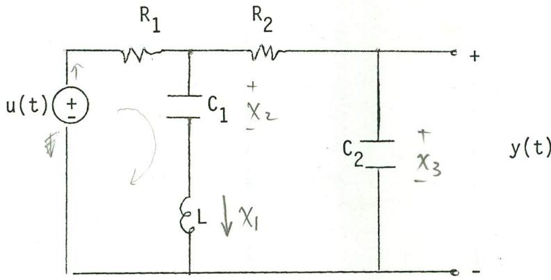
WLOG, Let  $R_1 = R_2 = 1$ ,  $C_1 = C_2 = 1$ ,  $L=1$ ,
