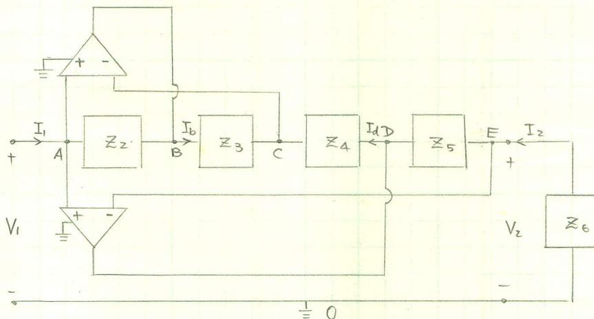
Apply the principle of virtual short circuit for both operational amplifiers.
