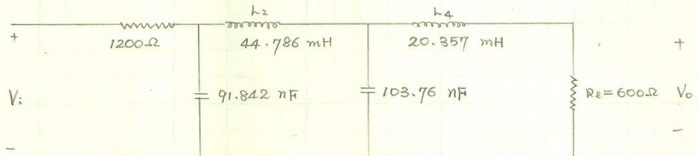
\* Replace the inductors in the circuit with GIC
