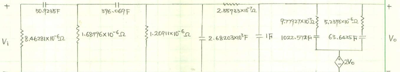
IMPEDANCE SCALING BY  $10^9$ , WE HAVE THE CIRCUIT REALIZATION:
