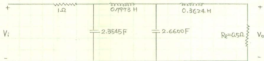
\* Scaling to the ripple bandwidth  $f_r = 3.4$  kHz,  $\omega_r = 2\pi f_r = 21362.83$  rad/s
