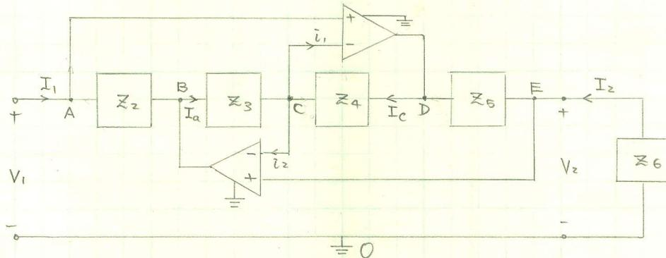
$$V_{AB} = I_1 Z_2, \quad V_{ED} = I_2 Z_5, \quad V_{CO} = V_{AO} = V_1, \quad V_{CO} = V_{EO} = V_2$$
