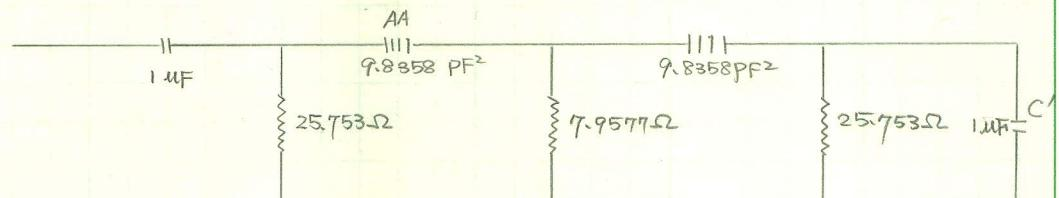
Using FDNR. with  $R_2 = R_3 = R_4 = 1K\Omega$ ,  $C_5 = 1\mu F$
