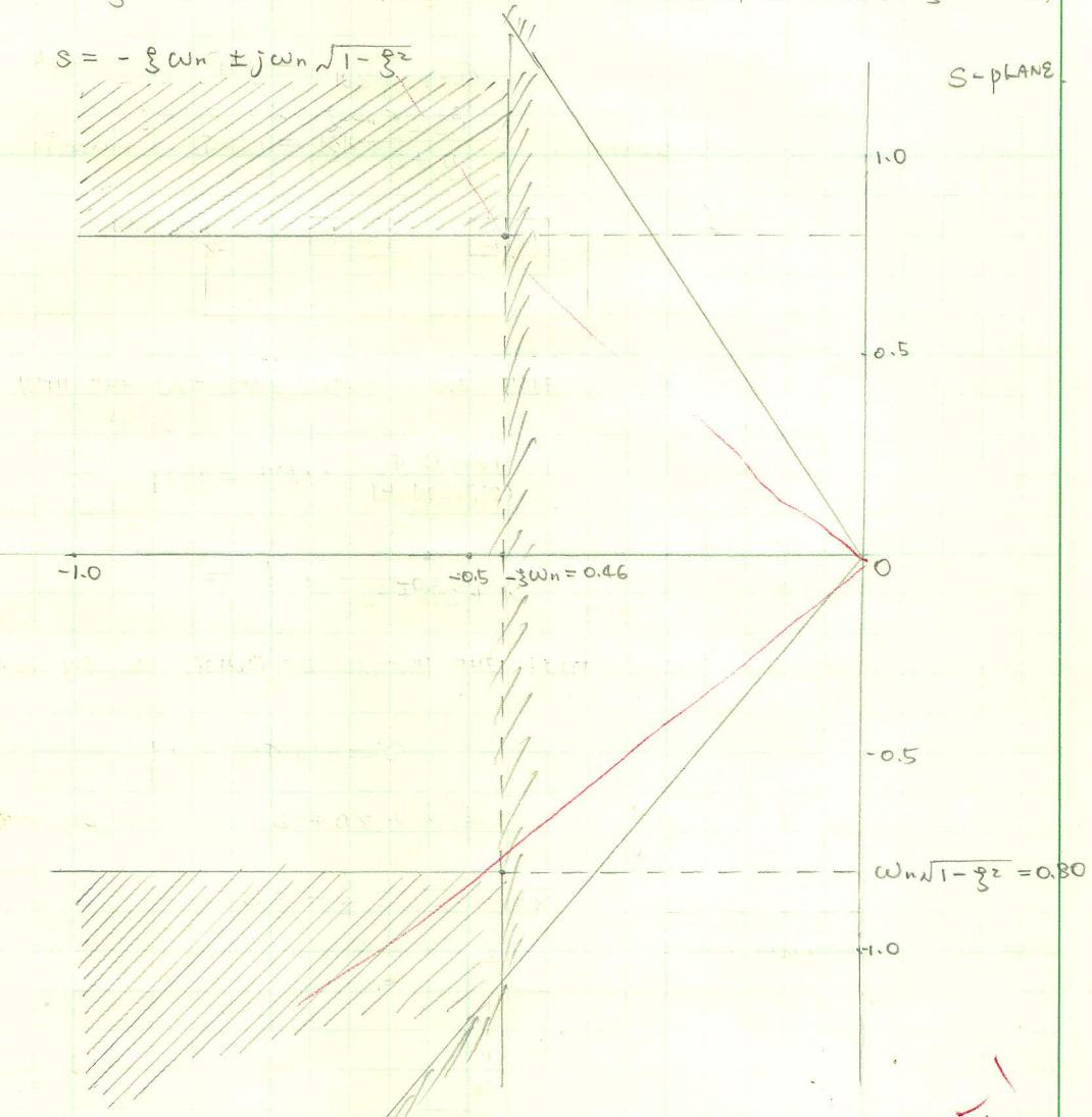
The following is the root locus on s-plane corresponding to the controller. (5.15)
