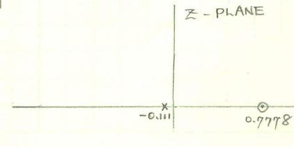
$$\text{ii) } H(z)|_{z=e^{j0.75}} = \frac{5(e^{j0.75} - 0.7778)}{e^{j0.75} + 0.1111} = 3.15143 / 54.90^\circ \quad \text{PHASE LEAD } 54.90^\circ$$
