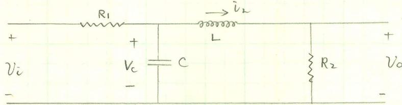
in term of  $R_1, R_2, L, C$  for the state variables  $v_c, i_w$ . Find the eigenvalue of the  $F$  matrix if
