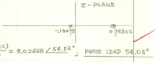
$$\text{ii) } H(z)|_{z=e^{j0.75}} = \frac{4.89259(e^{j0.75} - 0.76802)}{e^{j0.75} + 0.13498} = 3.02688 / 54.03^\circ; \quad \text{PHASE LEAD } 54.03^\circ$$
