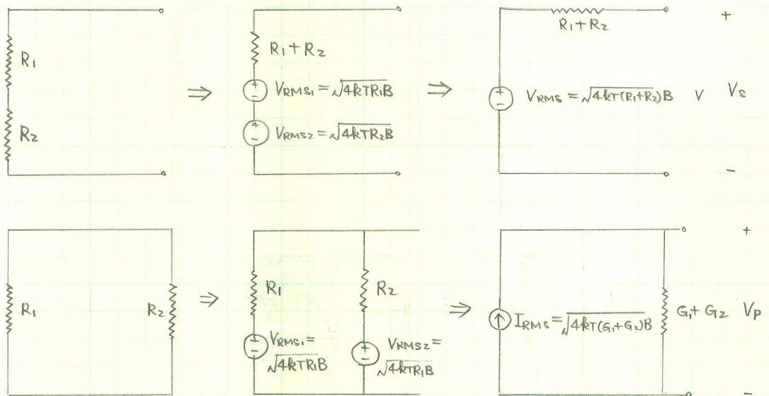
$$V_c = V_{RMS} = \sqrt{4kT(R_1+R_2)B}$$
