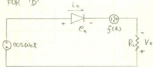
$$\begin{cases} i_1(t) = a_0 + a_1 e_1(t) + a_2 e_1^2(t) \\ i_2(t) = a_0 + a_1 e_2(t) + a_2 e_2^2(t) \\ i_3(t) = a_0 + a_1 e_3(t) + a_2 e_3^2(t) \\ i_4(t) = a_0 + a_1 e_4(t) + a_2 e_4^2(t) \end{cases}$$
