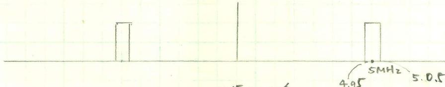
$$\overline{n_c^2(t)} = \overline{n_s^2(t)} = \overline{n^2(t)} = \frac{1}{\pi} \int_{4.95 \times 2\pi \times 10^6}^{5.05 \times 2\pi \times 10^6} 10^{-7} \left(1 - \frac{\omega}{2\pi \times 10^7}\right) d\omega$$
