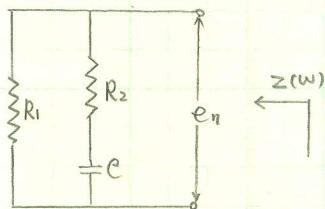
SOLUTION:  $z(w) = \frac{R_1 \cdot (R_2 + \frac{1}{j\omega C})}{R_1 + R_2 + \frac{1}{j\omega C}}$
