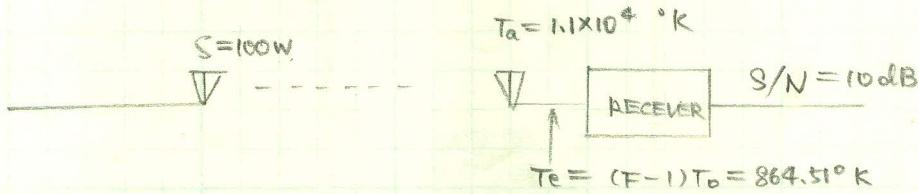
$N = k(T_a + T_e)B_N = 1.38 \times 10^{-23} (11000 + 864.51) \times 3 \times 10^3 = 4.91 \times 10^{-16} \text{ W}$
