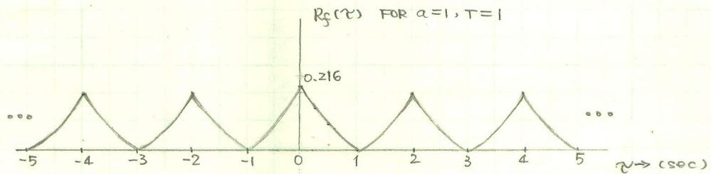
$$(b) \quad R_f(\tau) = \sum_{n=-\infty}^{\infty} R_n \cdot e^{jn\omega_0\tau}, \quad \text{WHERE} \quad \omega_0 = 2\pi/2T = \pi/T$$
