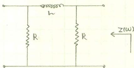
$$(a) \quad z(\omega) = R(R + j\omega L) / (ZR + j\omega L) = R(R + j\omega L)(ZR - j\omega L) / (4R^2 + \omega^2 L^2)$$
