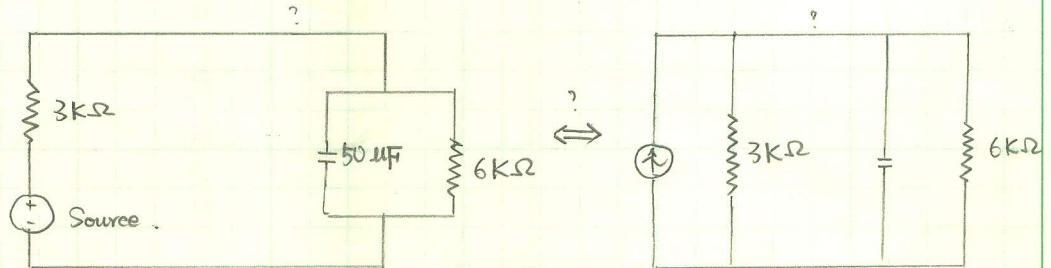
According to the circuit theorem, the mean power across the capacitor is zero.  $\therefore$
