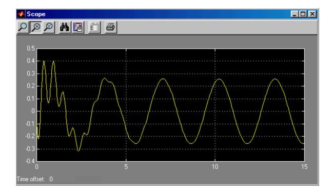
Transient response can be observed in the first few seconds. Eventually, the circuit settles down to the steady state response, which is a sinusoidal wave.
