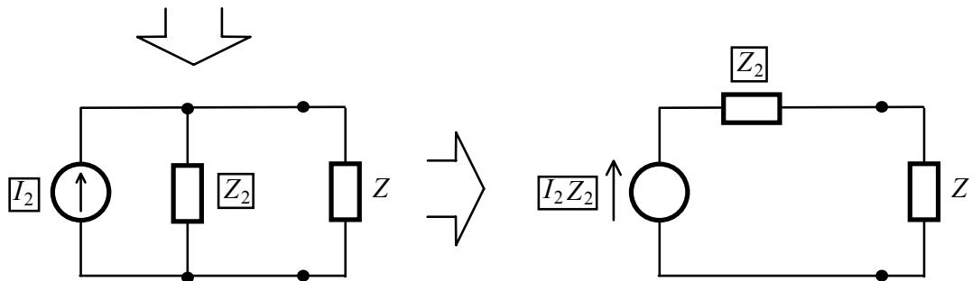
$$\begin{aligned} Z_2 &= -j25 \parallel 30 \parallel (10 + j15) = \frac{1}{\frac{1}{-j25} + \frac{1}{30} + \frac{1}{10 + j15}} = \frac{1}{\frac{1}{-j25} + \frac{1}{30} + \frac{1}{10^2 + 15^2}} \\ &= \frac{1}{0.0641 - j0.00615} = \frac{1}{0.0644e^{-j5.48^\circ}} = 15.5e^{j5.48^\circ} \end{aligned}$$
