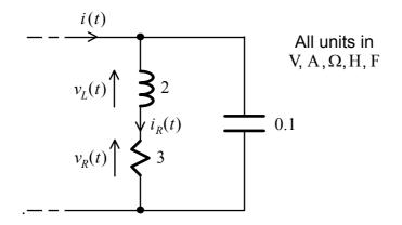
Determine  $i_R(t)$ ,  $v_L(t)$  and i(t) by using phasor analysis.
