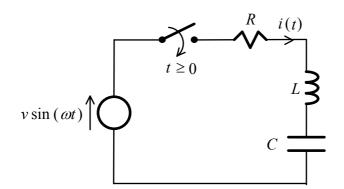
Derive the governing differential equation and initial conditions for finding the circuit current i(t) for  $t \ge 0$ . Determine the steady state current.
