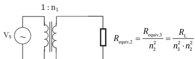
$$R_{\text{equiv}} = \frac{R_{\text{equiv},2}}{n_1^2} = \frac{R_L}{n_3^2 \cdot n_2^2 \cdot n_1^2} = \frac{100}{0.01^2 \cdot 0.1^2 \cdot 20^2} = 250000 \Omega = 250 \text{ k}\Omega$$
