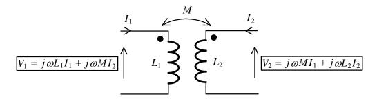
The primary and secondary inductances of the transformer are respectively given by
