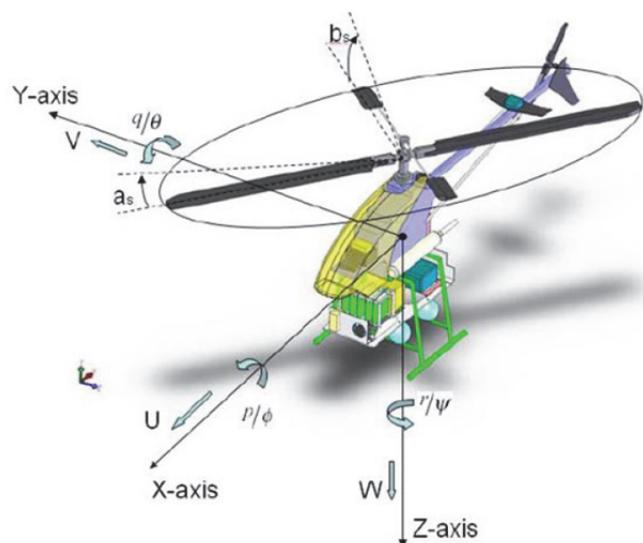
$U$ ,  $V$  and  $W$  are respectively the velocities of the chopper in the  $x$ ,  $y$  and  $z$ -axis of the body frame of the helicopter;  $\phi$  is the roll angle,  $\theta$  is the pitch angle, and  $\psi$  is the heading or yaw angle;  $p$ ,  $q$  and  $r$  are respec-
