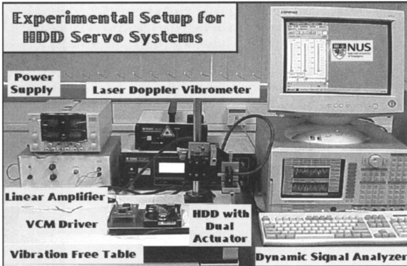
Figure 1.4. Implementation setup for HDD servo systems.
